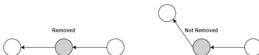
Figure 4.14: Image explanation of colinear points removal.
