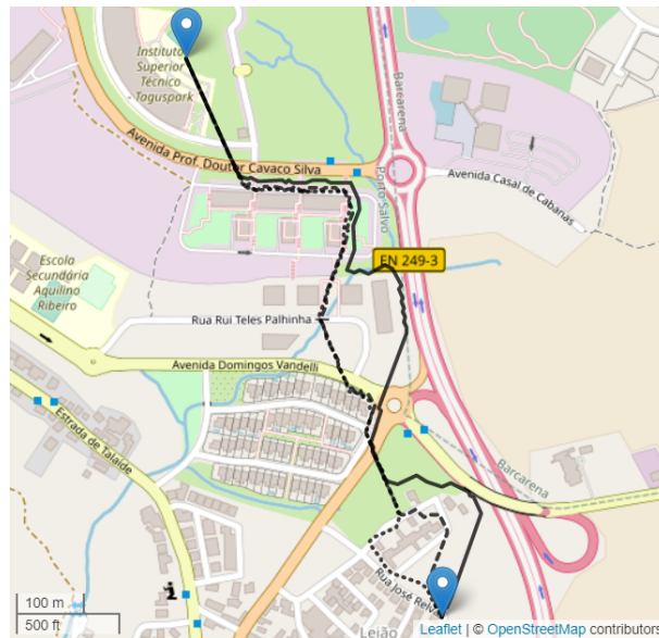
Figure 5.6: Path from IST Tagus to Location2, with distance between way-points: 1 meter with margin to buildings of 5 meters (dotted path); 2 meters with margin to buildings of 10 meters (dashed path); and, 5 meters with margin to buildings of 20 meters (solid path);.
