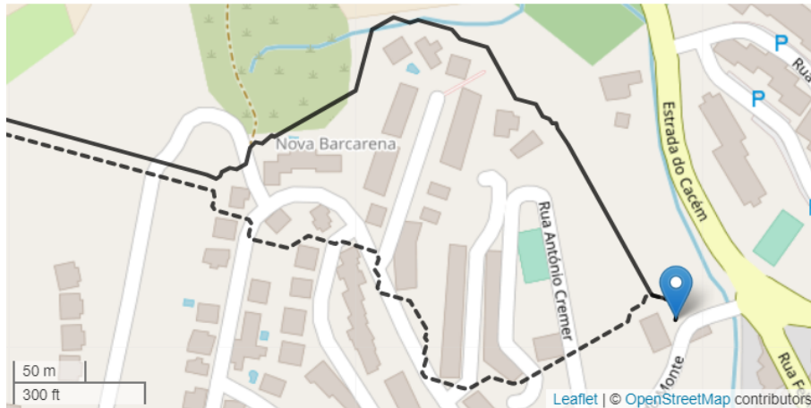
Figure 5.9: Final part's closeup of the trajectory from IST to Location1 mission, with resolution of 2 meters and margin to buildings of 10 meters. Online approach's path represented by the dashed line and Offline approach's path by the solid line.
