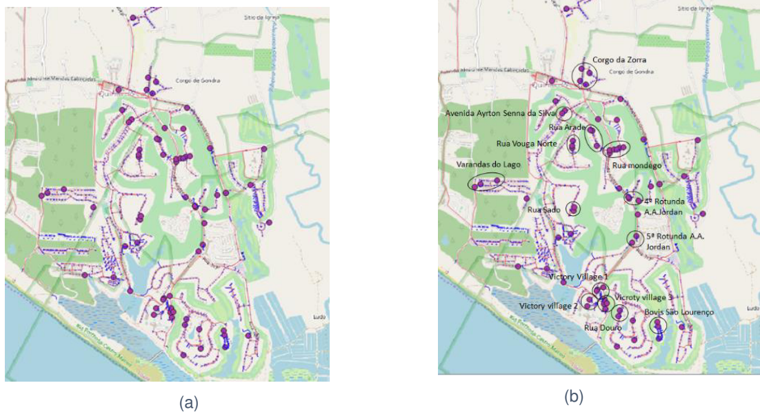
Figure 5-4 – Maps of distribution network: (a) Map of distribution pipe with failure location; (b) Map of distribution network with aggregated clustered.
