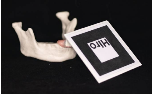
Figure 2.10: Fiducial marker use to enable the AR system to display the 3D model in the correct position.
