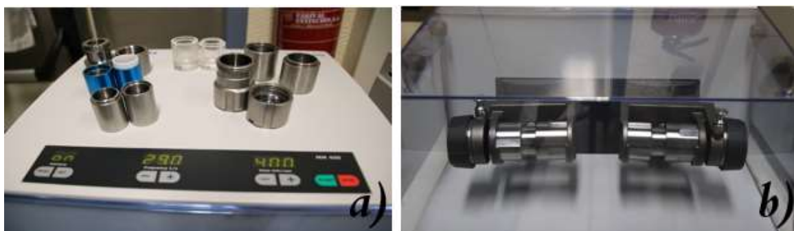
Figure 22: a) Different types of grinding jars that can be used for mechanochemistry b) Stainless-steel grinding jars in a Retsch MM400 ball mill
