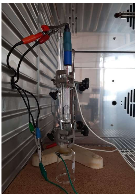
Figure 25: System of EIS inside an oven with controlled temperature and humidity
