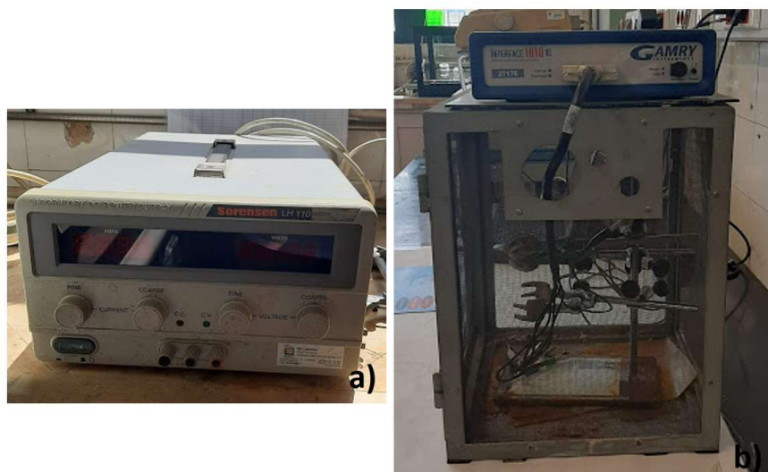
Figure 23: a) Laboratory DC Power Supply b) Gamry Interface on top couple to a Faraday cage
