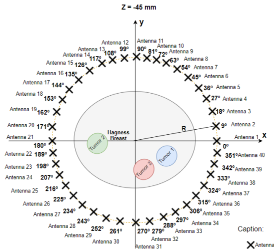
Fig. 7: All 40 XETS antennas around the Hagness breast phantom, where R is the distance between the center of the breast and the position of the antenna.
