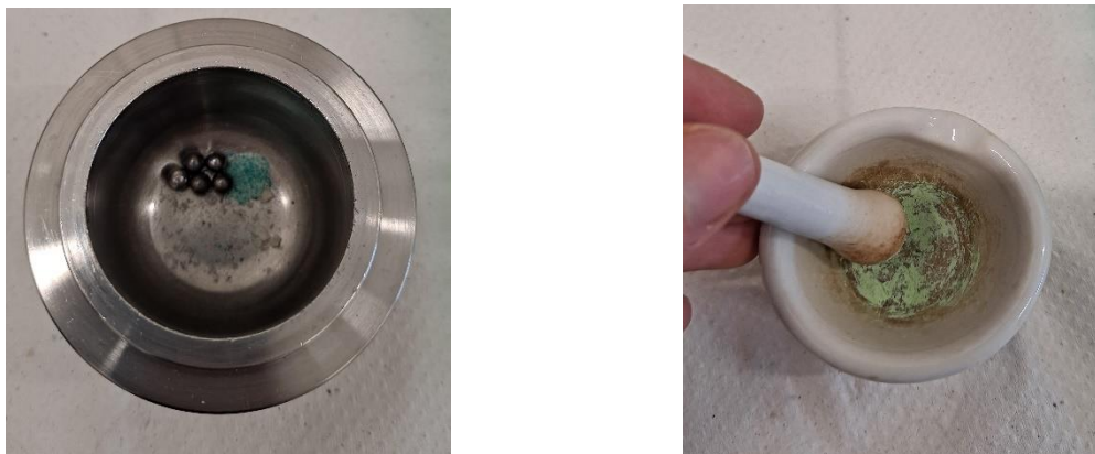
Figure 21: Grinding jar (Retsch® Planetary Ball Mill PM100) with reagents and spheres (left) and mortar (right).
