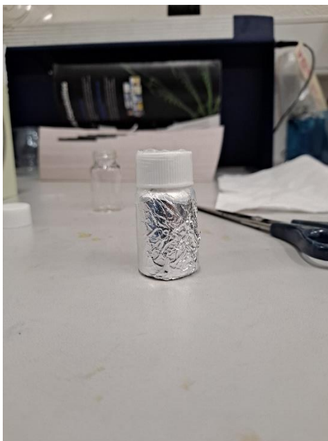
Figure 37: Light-protected flask that contains final reaction product from HMF microwave-assisted oxidation.
