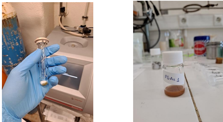
Figure 35: 10 mL vial for MW reaction (left) and collected final reaction product in flask for its refrigerated storage (right).
