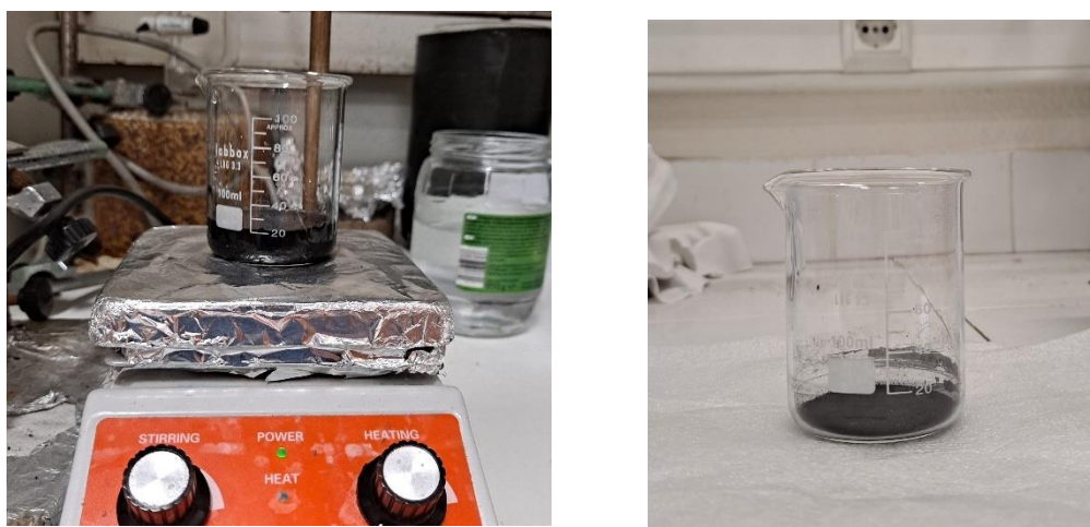
Figure 32: WI method: under continuous stirring (left) and after separation and dryness (right).
