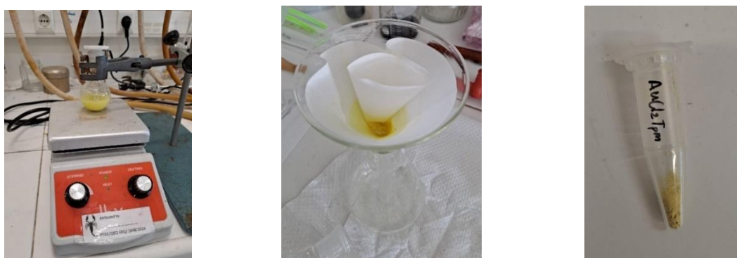
Figure 31: C-scorpionate gold(III) complex [\text{AuCl}_2(\text{Tpm})]\text{Cl} ( 4 ) traditional synthetic method.
