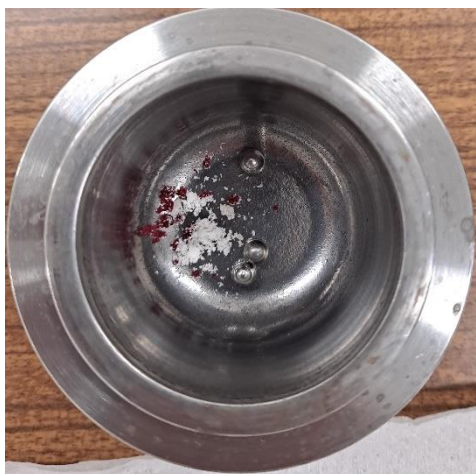
Figure 27: Grinding jar (Retsch® Planetary Ball Mill PM100) before (left) and after (right) ball milling of \text{CoCl}_2 \cdot 6\text{H}_2\text{O} + \text{Tpm} .
