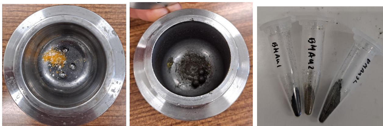
Figure 29: Grinding jar before (left) and after ball milling (centre) and the 3 first samples of C-scorpionate gold(III) complexes obtained by ball milling.
