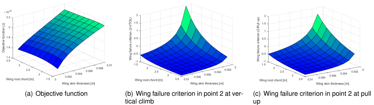
Figure 4.2: Behaviour of the real functions varying with the two design variables used in case 2.1
