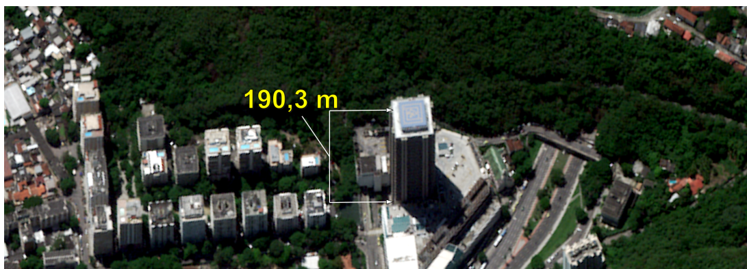
Figure 4.6: Building height measurement using SO CET GXP® (Rio de Janeiro, Brazil).
