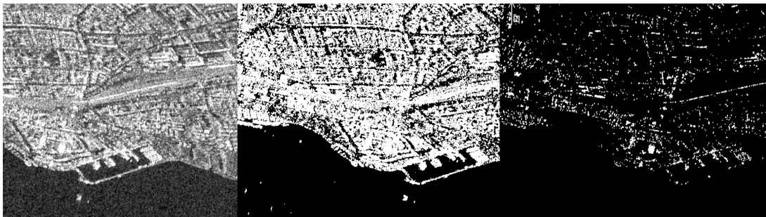
Figure 4.4: Threshold values at: 0 (left), 50 (center), 99 (right) using SO CET GXP® (Lake Constance, Germany).
