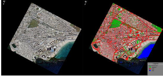
Figure 14: Supervised classification of vegetation, roads and water using SOCET GXP® (Tripoli, Libia).
