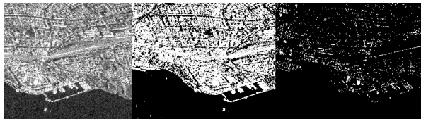
Figure 10: Threshold values at: 0 (left), 50 (center), 99 (right) using SOCET GXP ® (Lake Constance, Germany).
