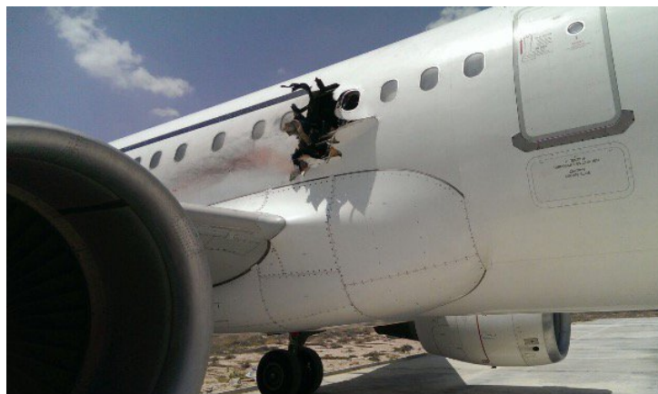
Figure 1.1: Result of the in-board explosion on Daallo Airlines flight 159 [2].
