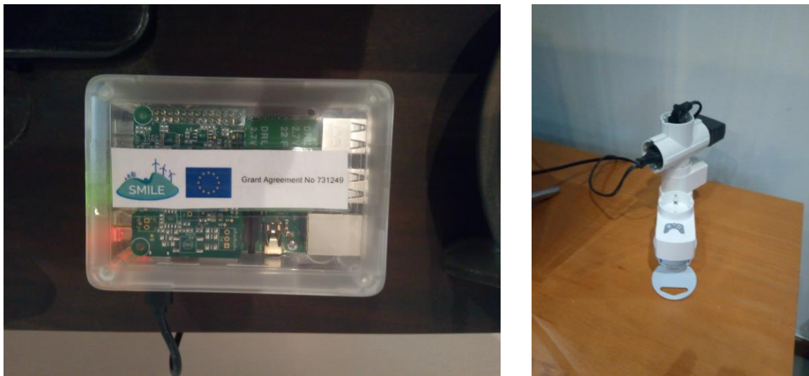
Figure 5.2 Individual appliance consumption collection setup: gateway (left), smart plugs (right)
