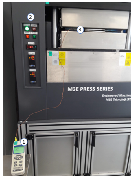
Figure 5.3: Hot Press Cure; 1- TM-947SD Thermometer, 2- Hot Press Panel; 3- Steel Plates
