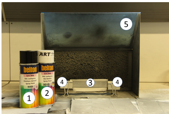
Figure 5.8: Speckle Pattern Paint; 1-Black Mate Paint, 2- White Mate Paint, 3- Sample Surface; 4- Grips, 5- Paint Box
