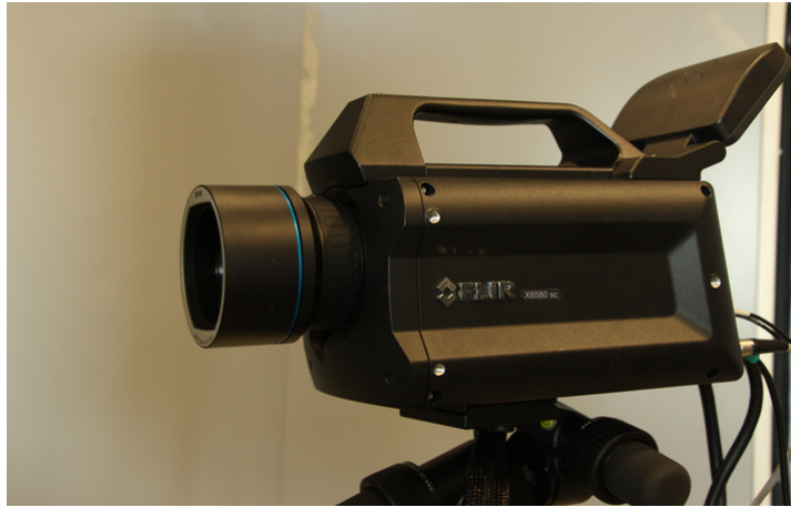
Figure 4.1: FLIR x6580sc infrared camera with 25 mm lens
