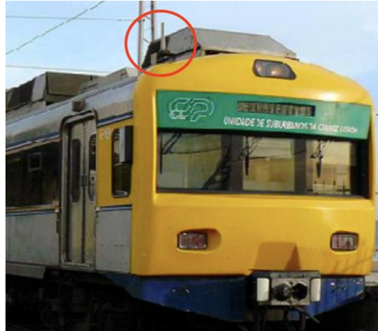
Figure 3.2 Elevated ground plane for antenna placement (adapted from [Sour13]).
