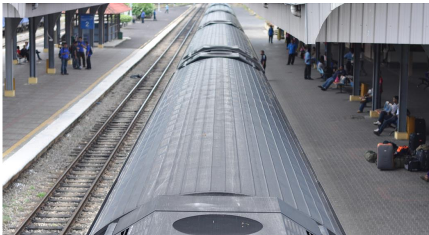
Figure 3.1 Longitudinal grooves on rolling stock roof (adapted from [Teoh09]).
