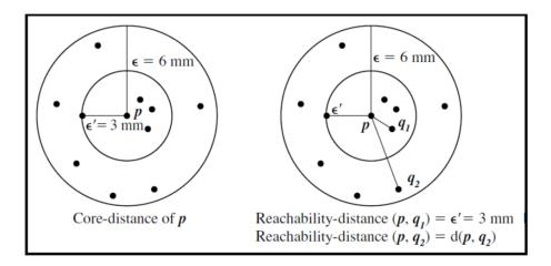
Figure 3.4: Illustration of core-distance and reachability-distance in OPTICS. Source: [40].
