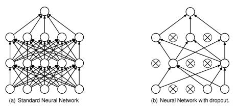
Figure 4.10: Application of dropout. Source:[49].
