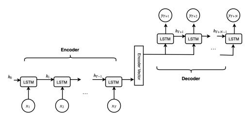
Figure 4.8: LSTM Encoder-Decoder.
