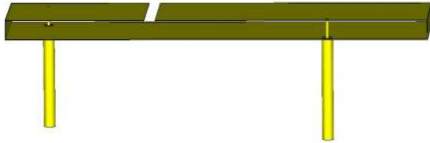
Figure 3.25: Optimal solution for position of the high band and low band ports placed at opposite positions with coaxial cables
