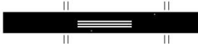
(b) Production mask for the photolithography process (ABViewer layout)
