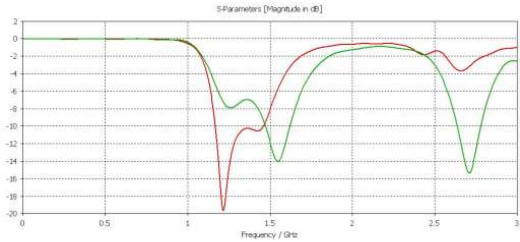
(a) Return loss of the low band port ( S_{22} )
