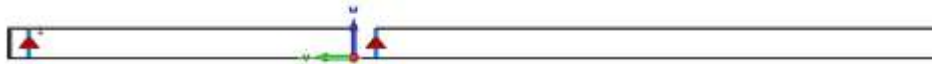
Figure 3.13: Example of position of the high band discrete port, fixing the low band one on the same side
