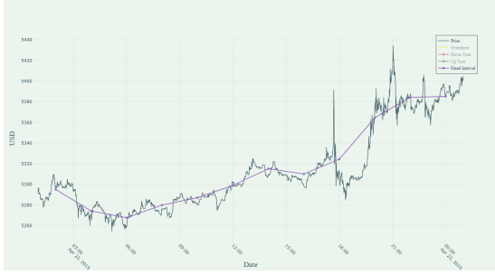
Figure 9: Price activities for BTC/USD on April 22, 2019. The blue line shows the tick-by-tick value of Bitcoin for that day. While the purple line is the fixed interval summary sampling the price value every two hours by means of averaging the asset value between a two hour window and stamping it to the right. This period is characterized by 11 intervals by the fixed physical time framework.
