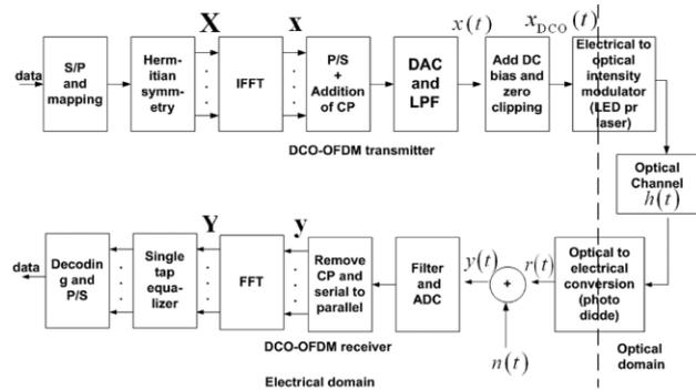
Fig. 2. Block diagram of an optical communication system using OFDM (adapted from [15]).
