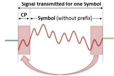
Fig. 4. Cyclic Prefix on an OFDM symbol.
