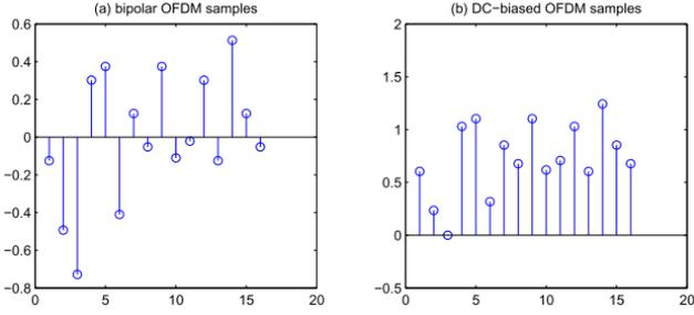
Fig. 5. Conversion of Bipolar OFDM to OFDM with DC component (adapted from [17]).
