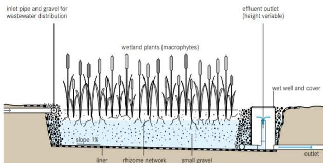
Figure 1: HSSF constructed wetland
