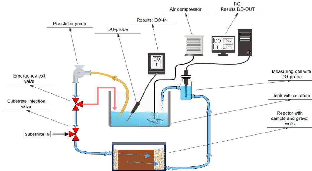
Figure 4: Representation of the LSF respirometer test setup
