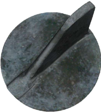
Figure 5: 3D scan image of the anode after the test
