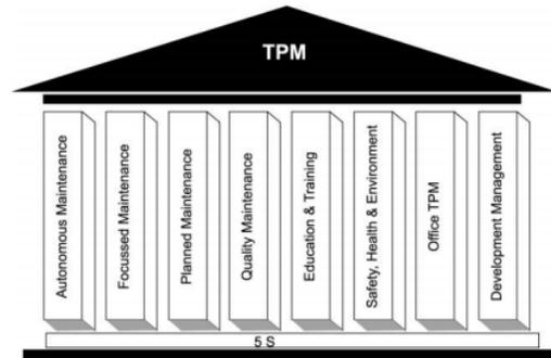
Figure 2: TPM Pillars suggested by JIPM, Ahuja et al. (2008).
