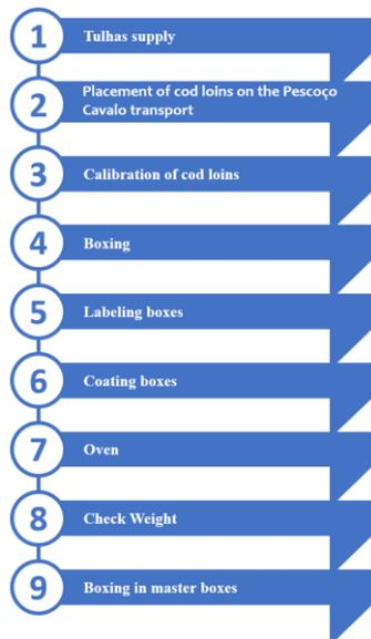
Figure 4: Packaging process of line 1.
