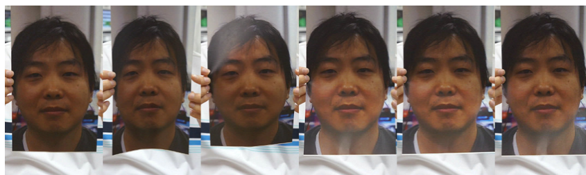
Figure 2.3: Example sequence of a warped photo attack from the CASIA Face Anti-Spoofing Database. [12]
