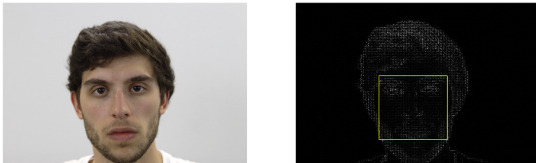
Figure 3.5: Original image and its HOG transformation, capturing the major features of a face.
