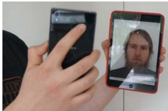
Figure 2.2: Spoofing attack with a hand-held photo, also referred to as a digital-photo attack. [11]
