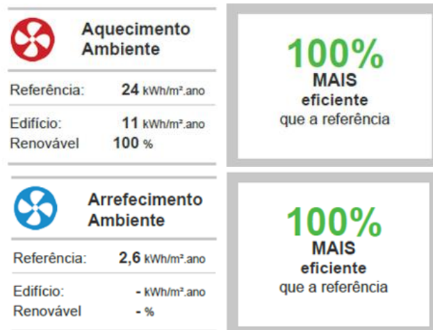
Figure 11. Heating and cooling energy requirements and share of energy from renewable sources
