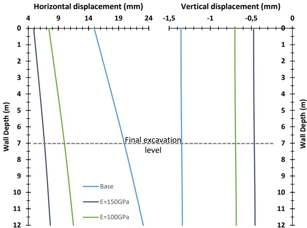
**Figure 40 - Vertical and horizontal displacements for the different values of the soil stiffness.**
