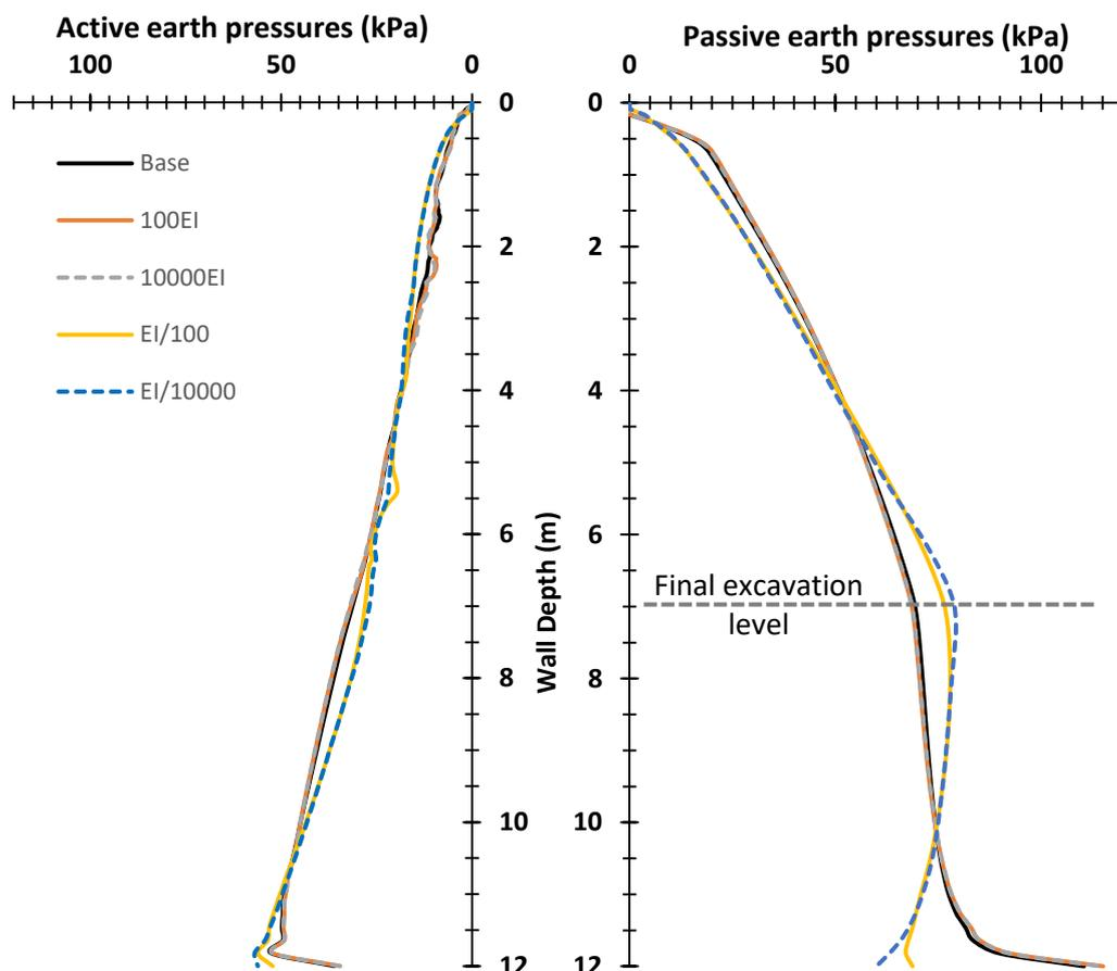
**Figure 35 - Earth pressures for different values of wall stiffness (left side – active, right side – passive).**
