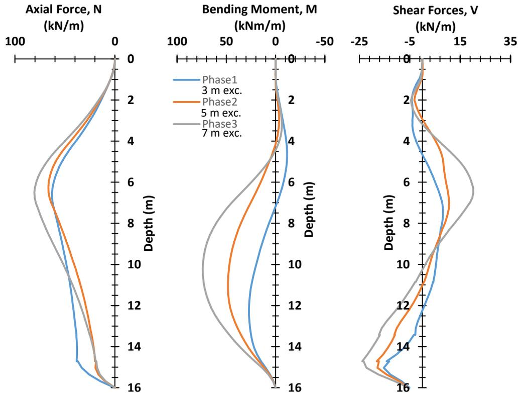
**Figure 48 – Wall forces for three excavation phases of the base model**
