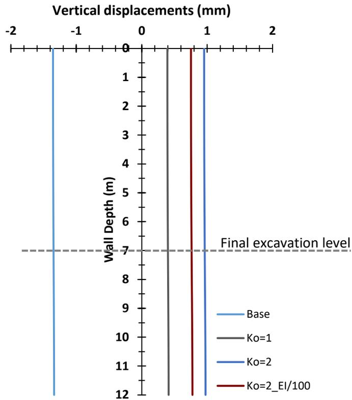
Figure 45 - Vertical displacements for the different values of the  $K_o$ .
