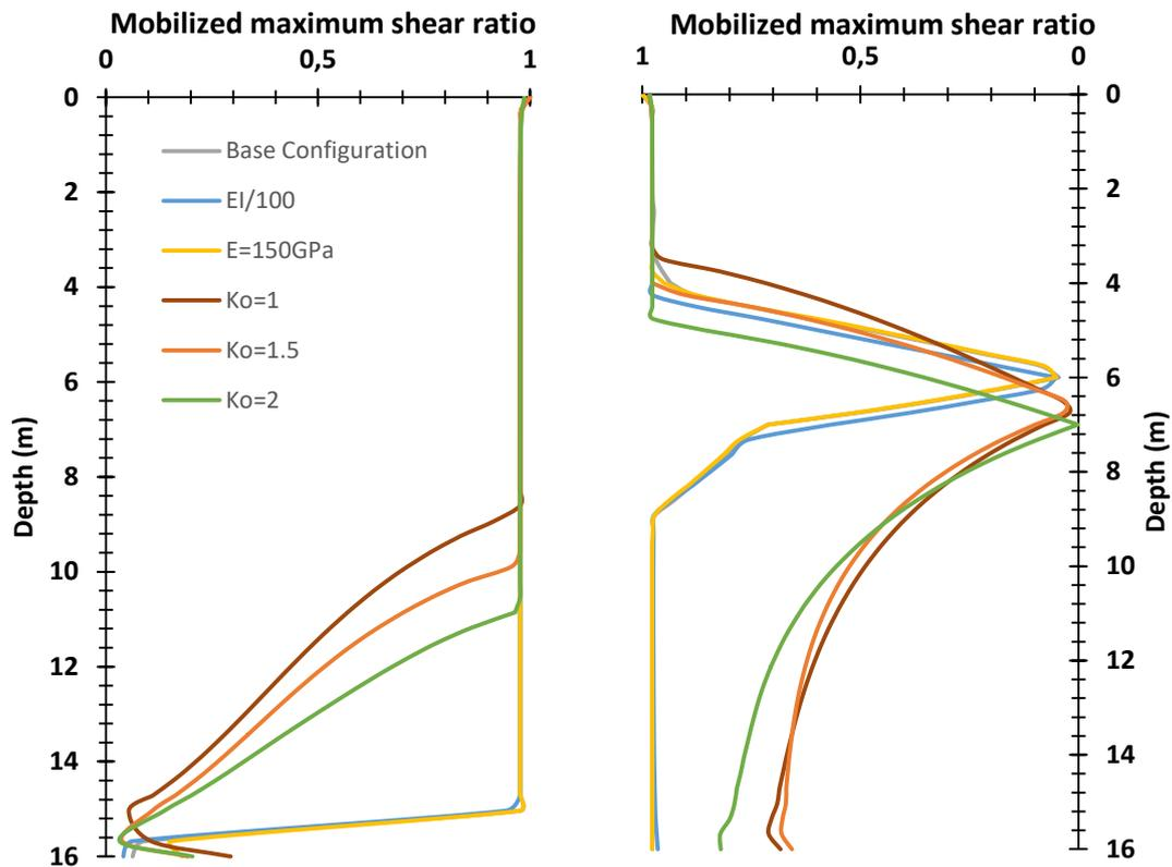
Figure 55 - Relative shear stresses for the different configurations.
