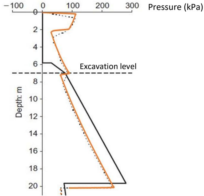
**Figure 10 - Comparison of effective earth pressure distributions using MCW method.**
