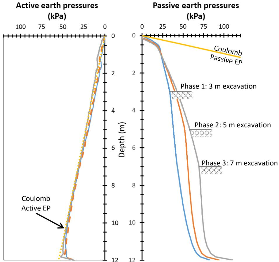
**Figure 26 - Base analysis – Development of earth pressures during berm formation**
