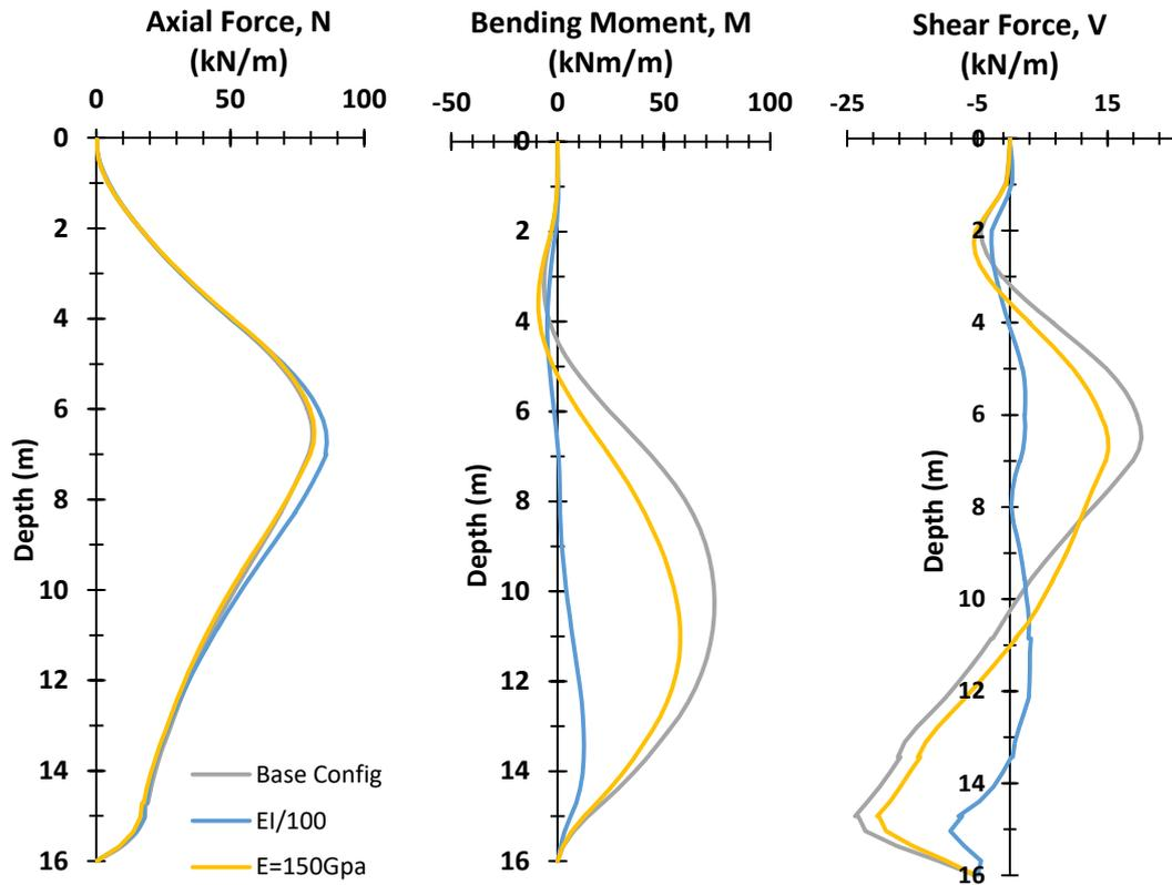
Figure 52 - Forces in the wall for different values of the soil stiffness and wall stiffness.
