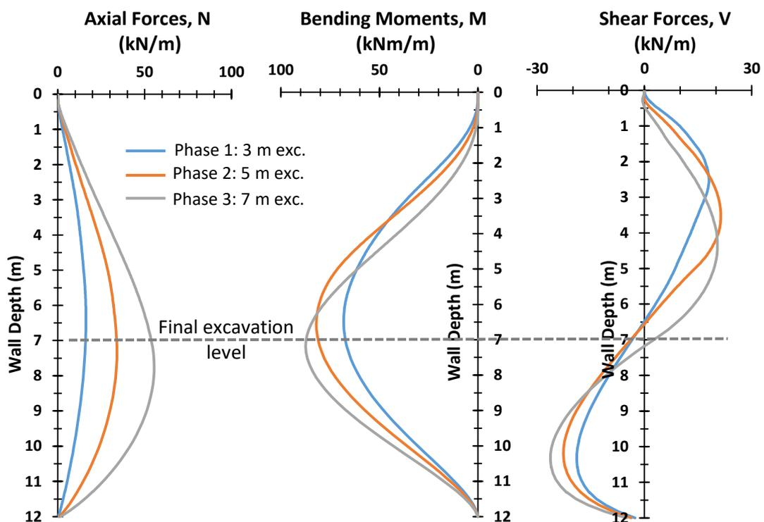
Figure 29 - Force distribution in the wall.
