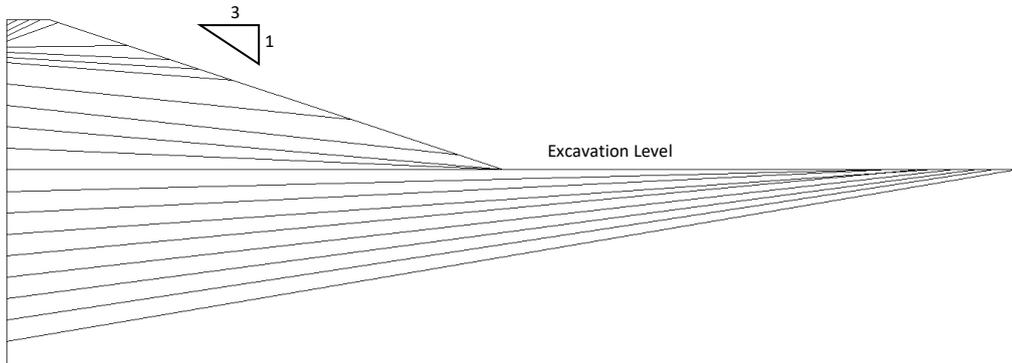
**Figure 22 - Critical slip surfaces for 3H:1V berm.**
