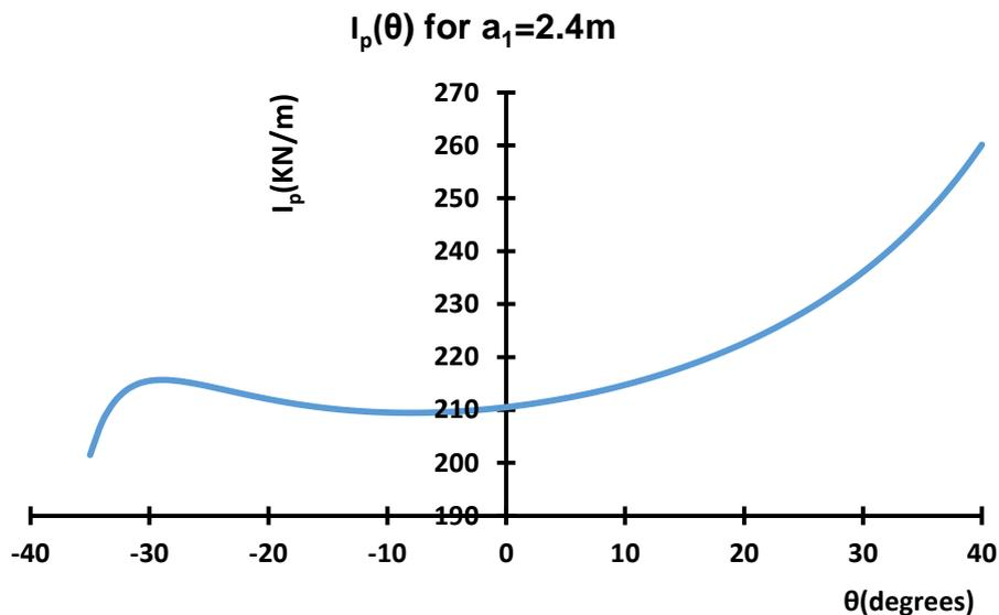
**Figure 68 - Critical angle  $\theta$  against  $I_p$  chart for the depth of 2.4 m.**
