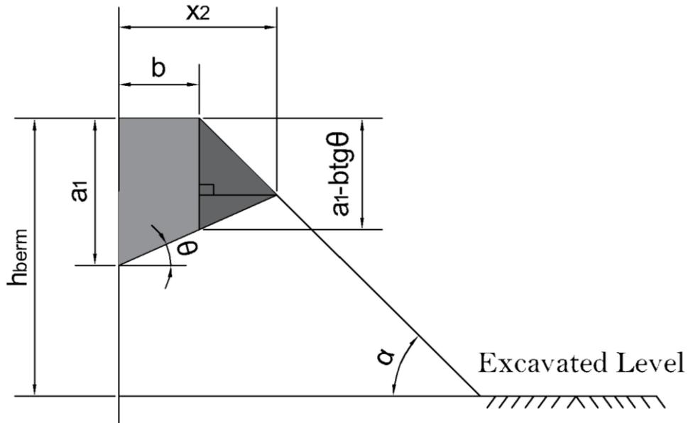
**Figure 62 - Area of the wedge inside the berm.**
