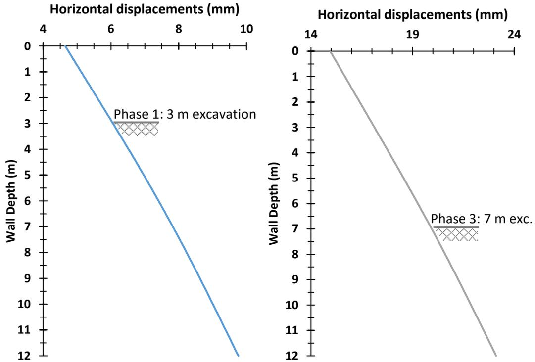
Figure 30 - Horizontal displacements of the wall for the 1<sup>st</sup> and 3<sup>rd</sup> excavation phases.
