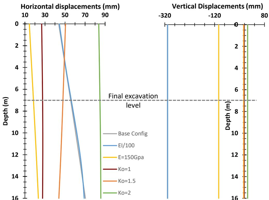
**Figure 54 - Wall displacements for different configurations.**
