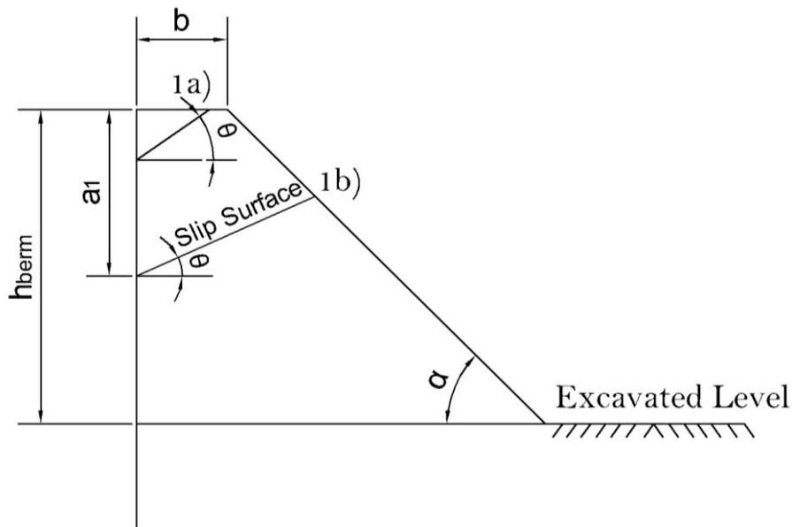
**Figure 60 - Slip surfaces inside the berm**
