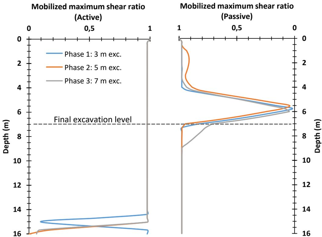
Figure 50 - Relative shear stresses for the three excavation phases of the base model
