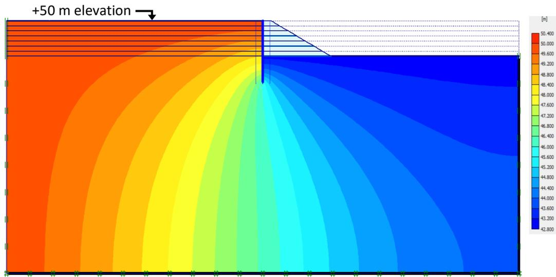
Figure 27 - Pore water pressure contours.
