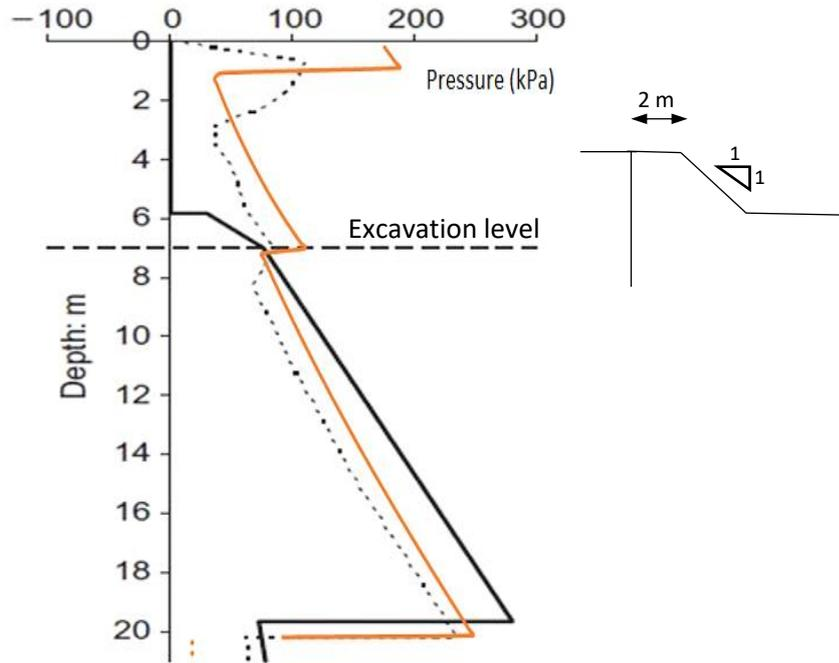
**Figure 14 - Earth pressure distributions for 1H:1V berm with 2 m wide top bench with suctions.** MCW earth pressures from Smethurst & Powrie, 2007 are dashed black line; REF, solid black lines; orange lines, this work.
