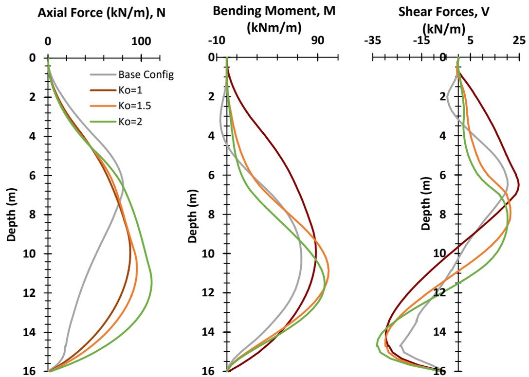
Figure 53 - Forces in the wall for different values of  $K_o$ .
