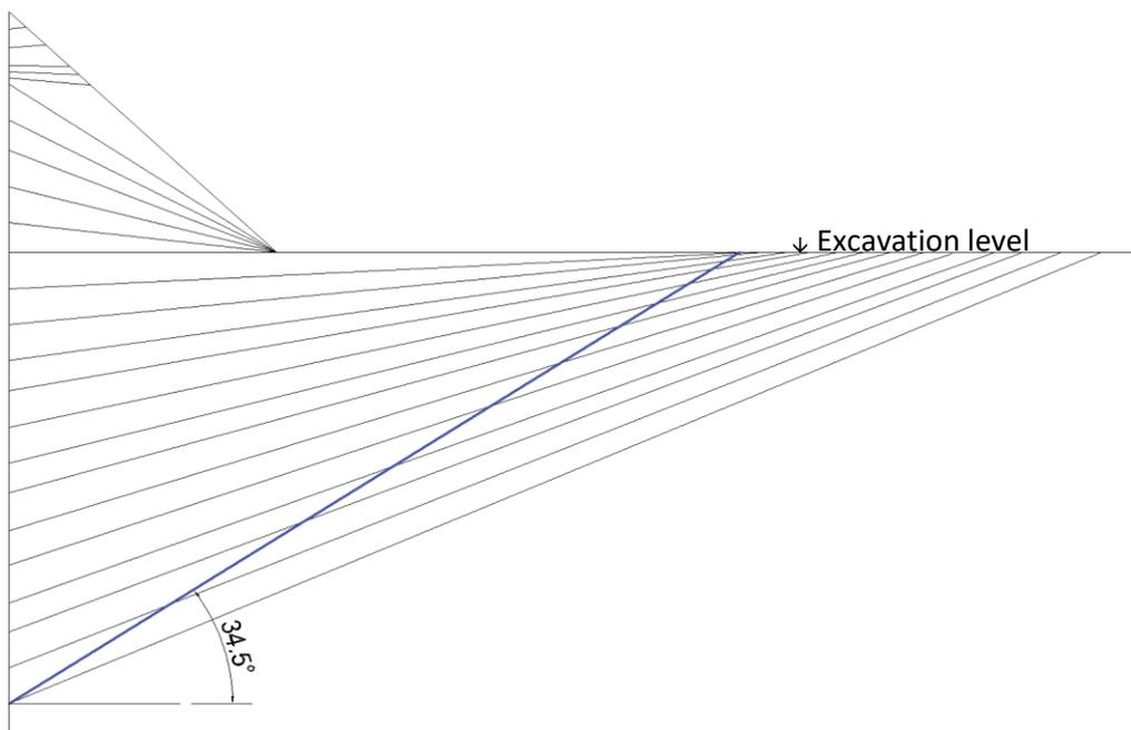
**Figure 13 - Critical slip surface locations from MCW method, with Coulomb slip surface (blue line)
