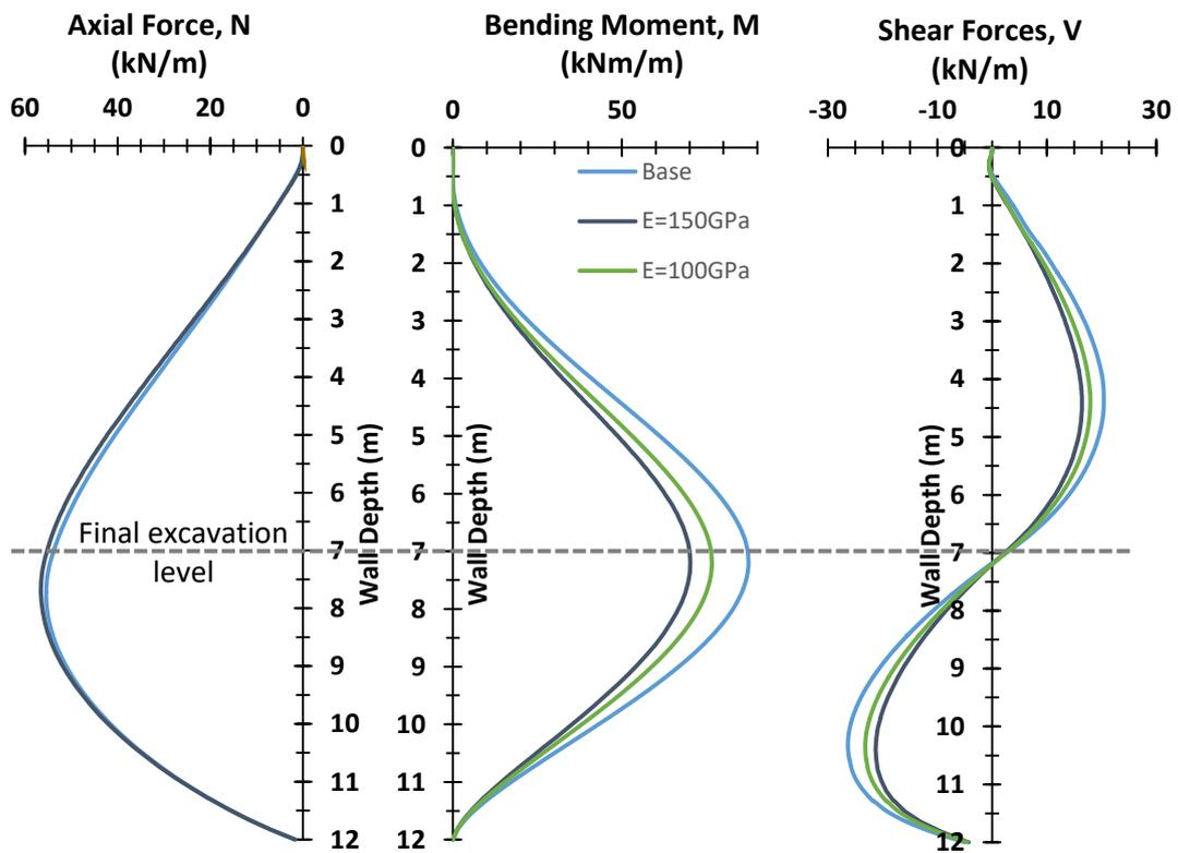
Figure 39 - Forces in the wall for different values of soil stiffness.
