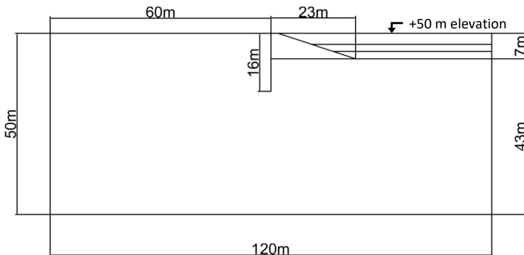
Figure 46 - Dimensions of the 3H:1V model.
