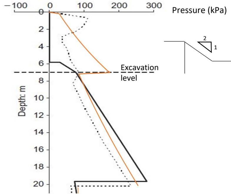
**Figure 16 - Effective earth pressure distributions for 2H:1V berm with no suctions.**
