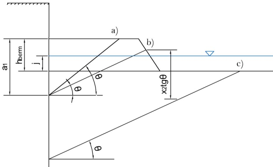
**Figure 66 - Three different situations of the slip surface.**
