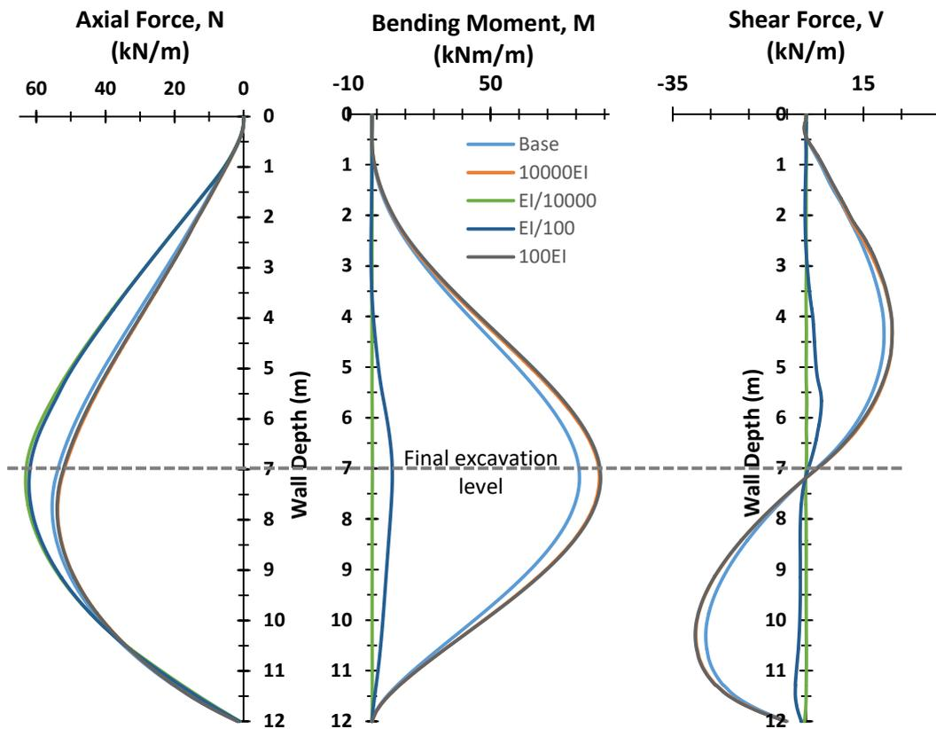
**Figure 36 - Forces along the wall for different values of wall stiffness.**
