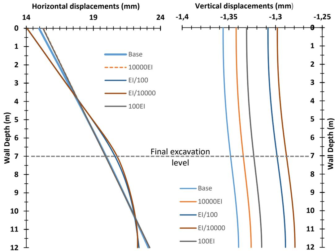
**Figure 37 - Horizontal and vertical displacements for different wall stiffness values, at final excavation level and berm fully formed.**
