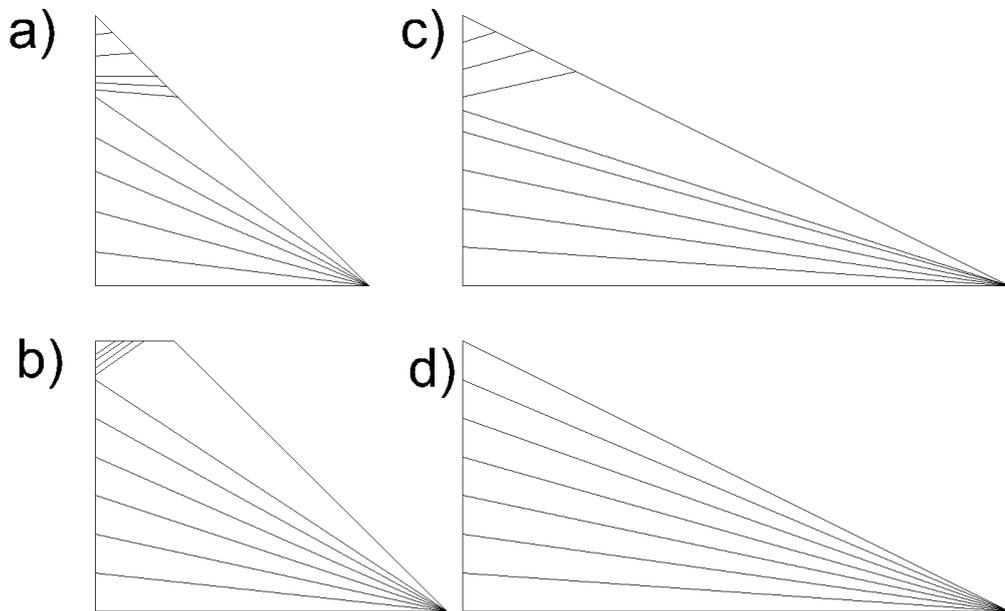
**Figure 17 - Critical slip surfaces for differing berm configurations.**
