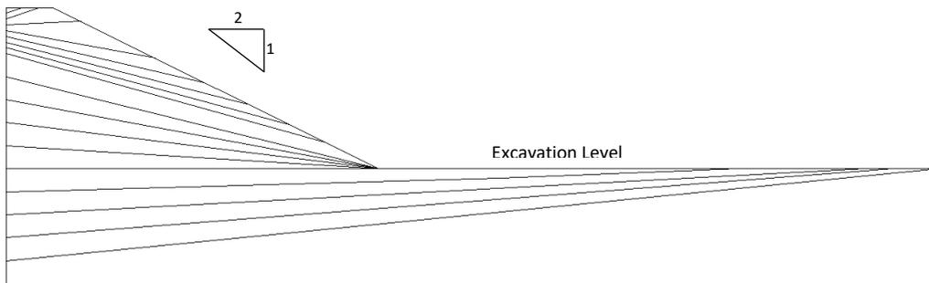
**Figure 20 - Critical slip surfaces for 2H:1V berm.**
