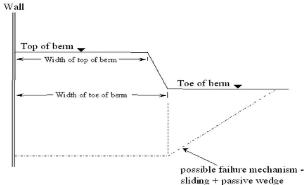
**Figure 6 - Failure mechanism for WALLAP Step 1, Part 4) mechanism.**
