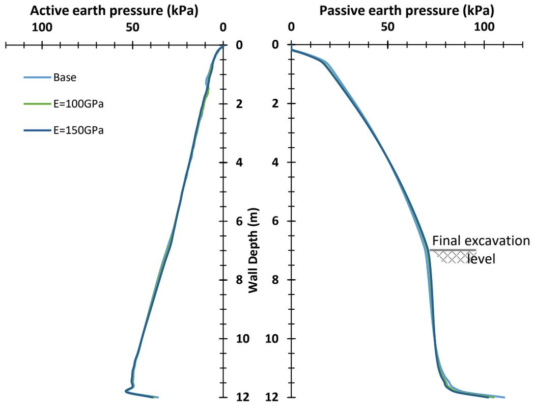
Figure 38 - Earth pressures for different values of soil stiffness
