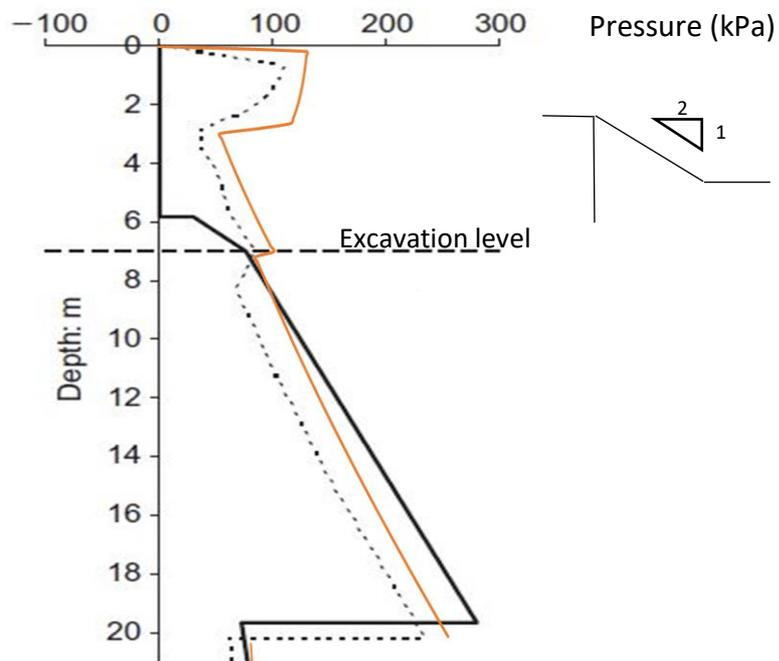
**Figure 15 - Effective earth pressure distributions for 2H:1V berm with no top bench with suctions.** MCW earth pressures from Smethurst & Powrie, 2007 are dashed black line; REF, solid black lines; orange lines, this work.
