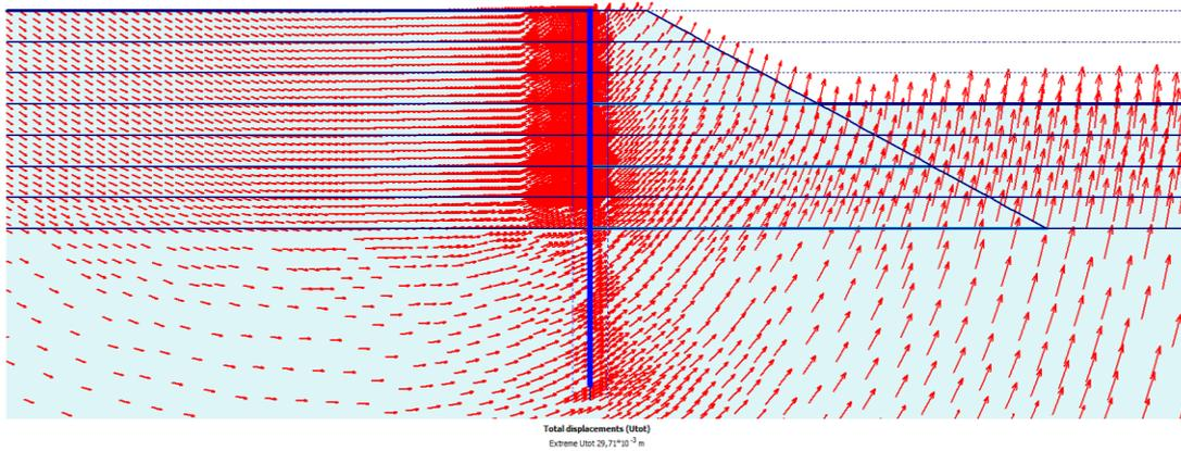
**Figure 33 - Total displacement field for the 1<sup>st</sup> phase.**
