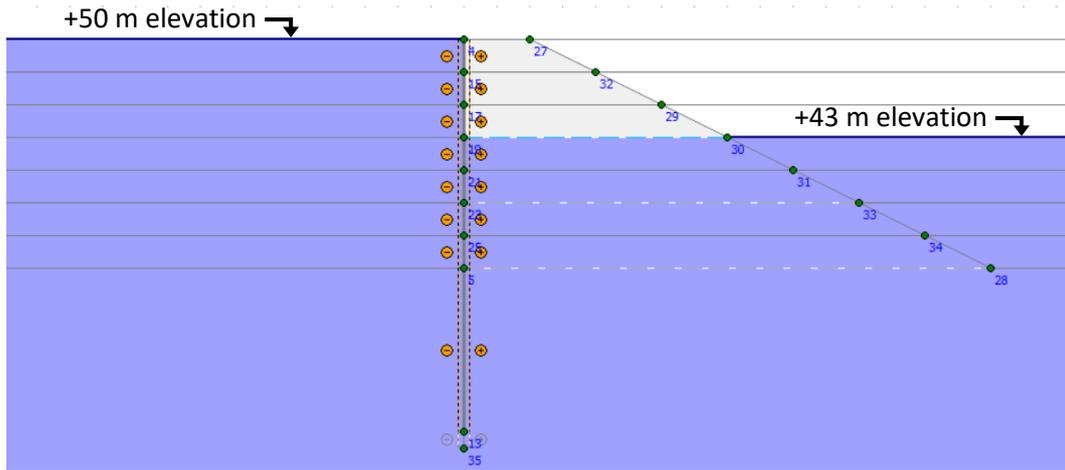
Figure 24 – Stage 1 of FEA - insertion of drains to maintain dry berm assumption (blue dash line - active; white dash - inactive).
