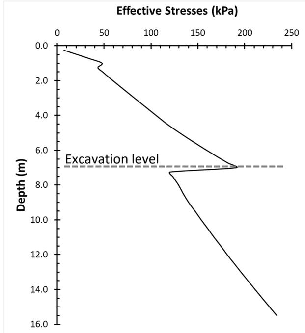
**Figure 21 - Effective earth pressure distributions for 3H:1V berm.**
