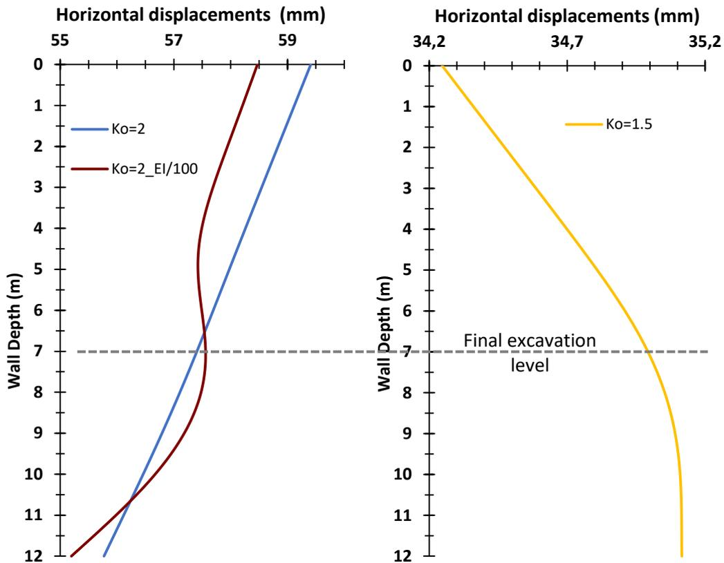
**Figure 44 - Horizontal displacements for the different values of  $K_0$  with amplified scale.**
