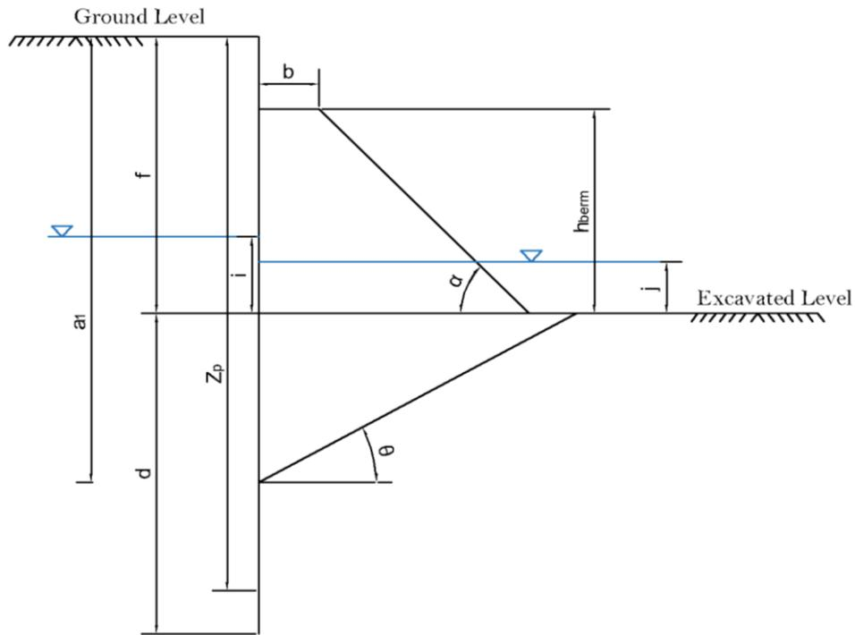
Figure 58 - Schematic representation of the berm geometry.
