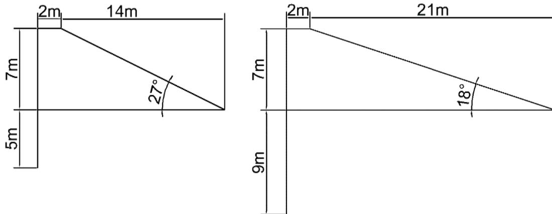
Figure 18 - Berm configuration.
