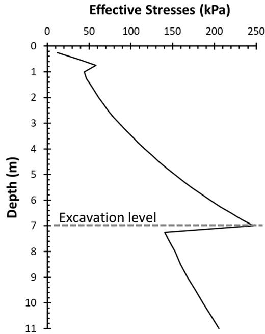
**Figure - 19 Effective earth pressure distributions for 2H:1V berm.**
