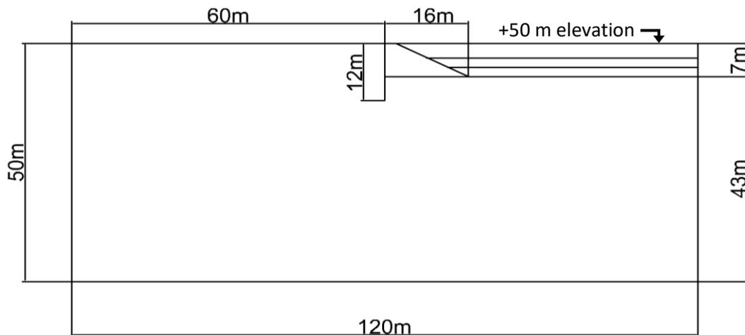
*Figure 25 - Dimensions of 2H:1V berm model.*
