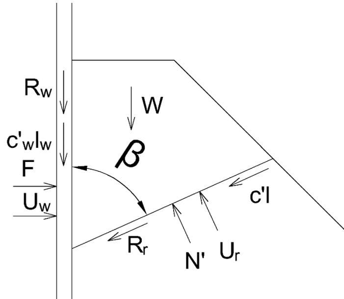
**Figure 59 - Forces acting on the wedge.**
