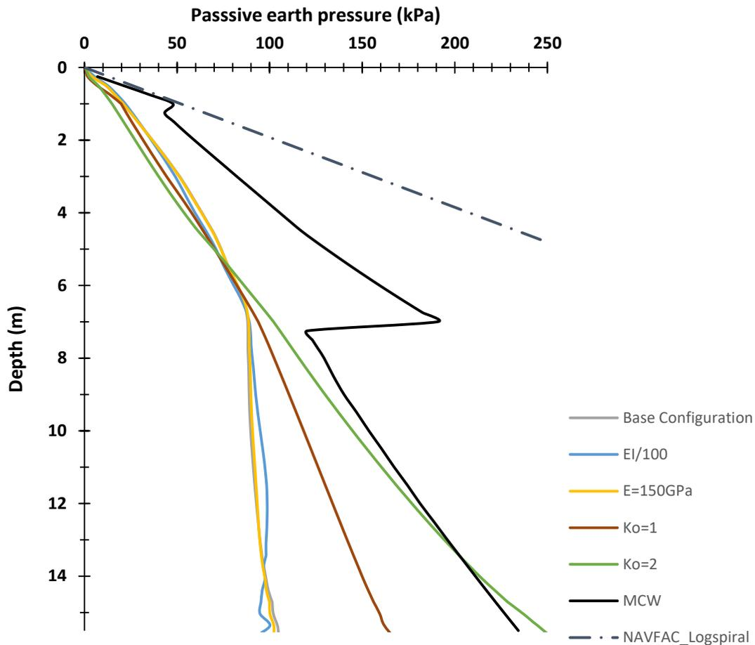
**Figure 57 - Effective passive pressures of the 3H:1V geometry obtained by the different methods and configurations (FEA).**
