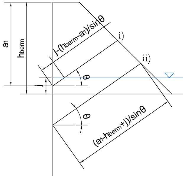
**Figure 67 - Slip surfaces for the different  $l^*$  calculation.**
