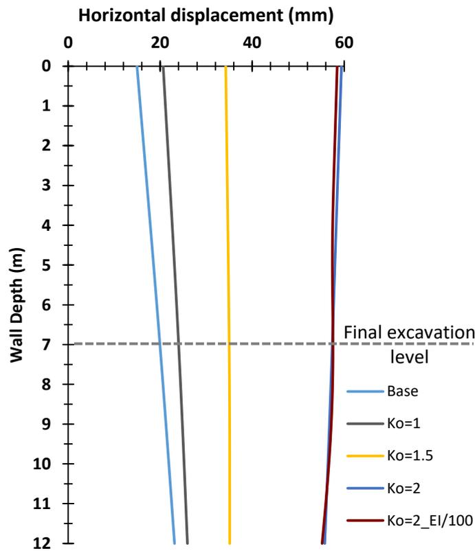
Figure 43 - Horizontal displacements for the different values of  $K_o$ .
