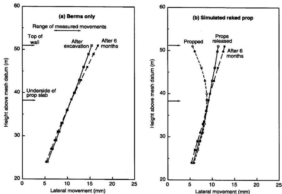
**Figure 1 - Lateral movements of the wall obtained by the FEA for the berm supported excavation and the propped excavation, Easton & Darley (1999).**
