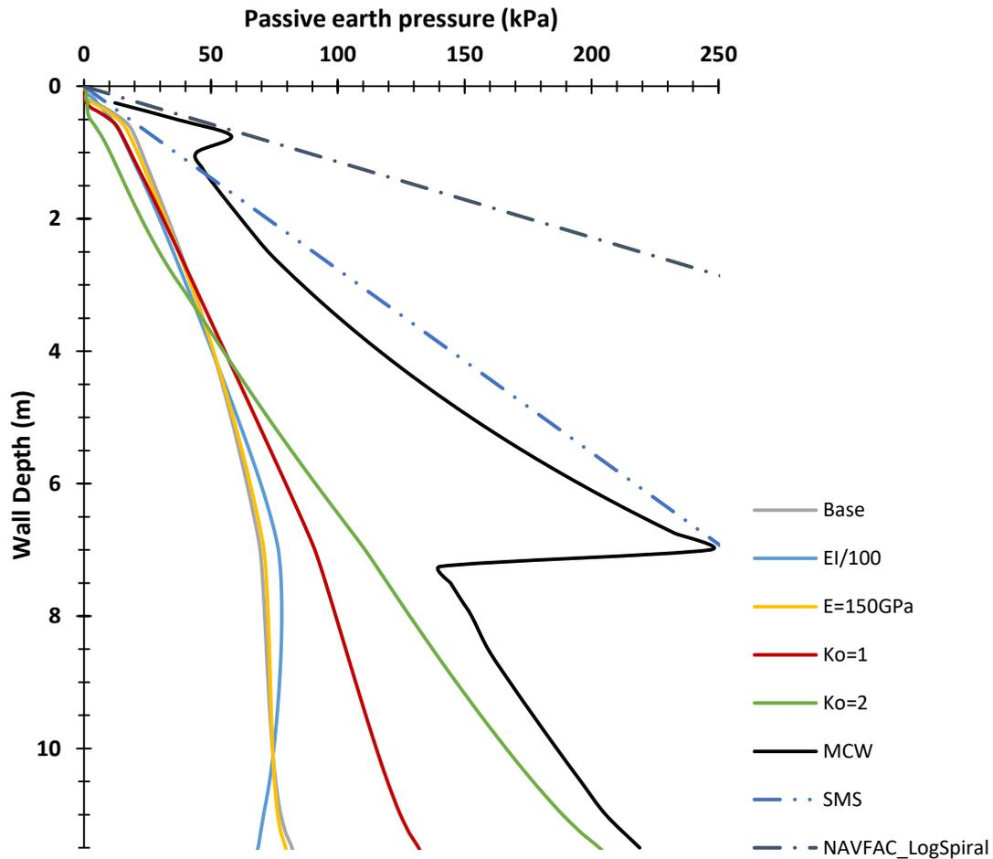
**Figure 56 - Effective passive pressures of the 2H:1V geometry obtained by the different methods and configurations (FEA).**
