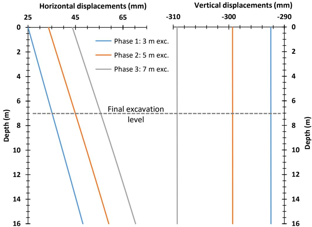
**Figure 49 - Total displacements of the three excavation phases for the base model.**
