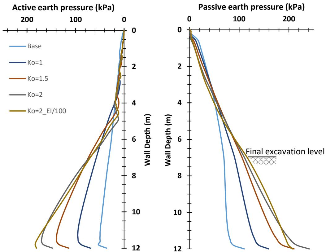
**Figure 41 - The earth pressures for the different values of  $K_o$**
