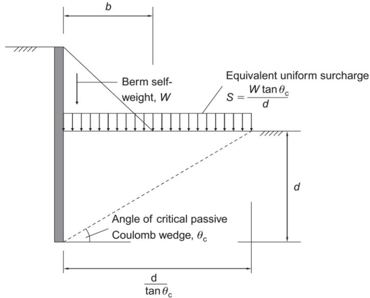
**Figure 4 - Schematic representation of the ESM method, Smethurst & Powrie (2008)**
