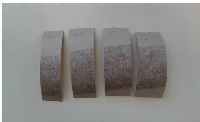
Fig. 3. Rips of paper glued by bio-based polyurethane adhesives.
