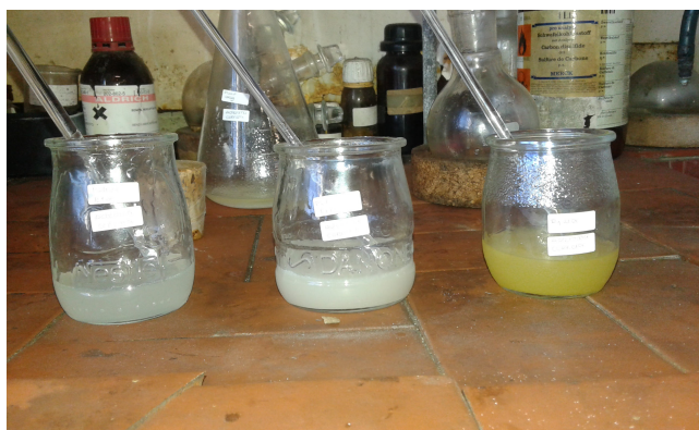
Fig. 4. Polyols obtained from NCO, UCO and VCO, from left to right
