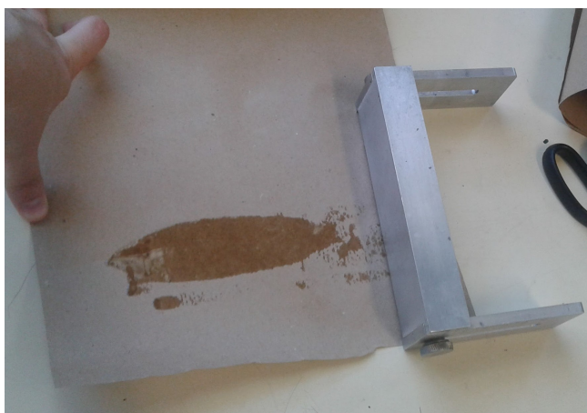
Fig. 2. Application of the polyurethane adhesives at the test paper.
