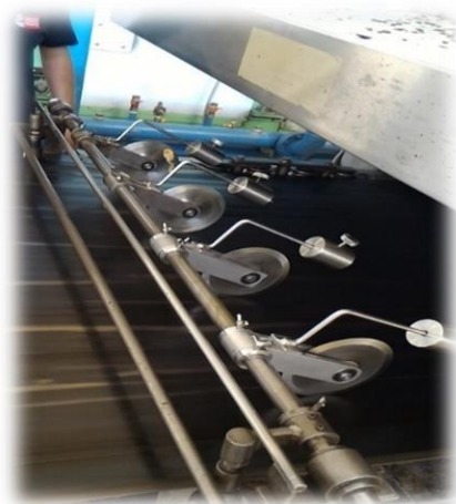
Figure 11 - Real image of the improvement implemented in dough cutting
