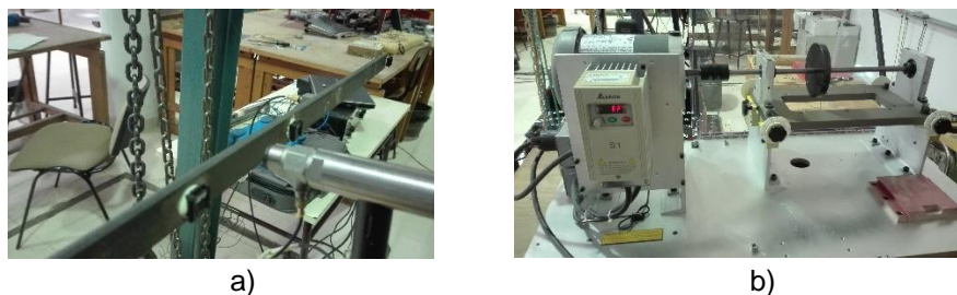
Figure 3 – Experimental models: a) Steel Beam suspended on a portal crane; b) SpectraQuest's Machinery Fault Simulator (MFS) used for resonance test.
