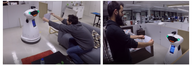
Fig. 7. Robot in a real world benchmark, on the mission domain situation, with a real human giving external sensor information with a QR code. On the left, the robot is in the sofa location and on the right the robot is in the bed location.
