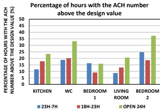
Figure 7 - PHAD for the cooling season (simulations performed without using fixed openings for ventilation in the facades)
