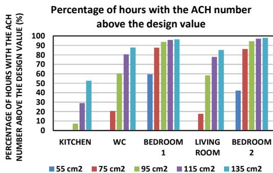
Figure 11 - PHAD in the heating season for the simulations performed using the wind speed according to the *Weather file*
