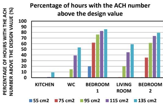
Figure 15 - PHAD in the heating season for the simulations performed using zero wind speed
