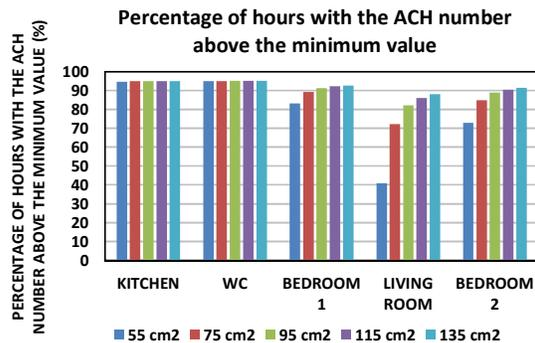
Figure 16 - PHAM in the heating season for the simulations performed using zero wind speed
