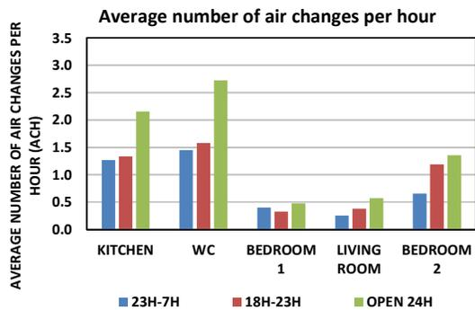
Figure 6 - Average ACH for the cooling season (simulations performed without using fixed openings for ventilation in the facades)
