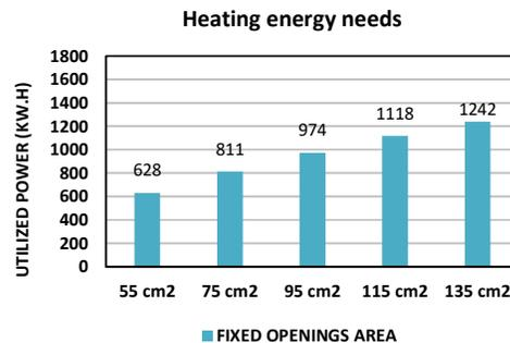
Figure 17- Heating energy needs for the simulations performed using zero wind speed, in the heating season
