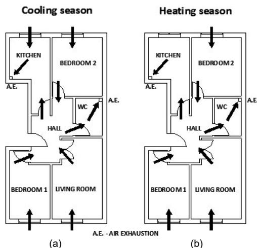
Figure 2 – Ventilation scheme of the model for the conventional cooling season (a) and conventional heating season (b)
