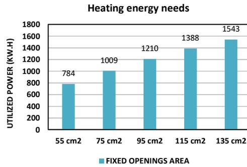
Figure 13 – Heating energy needs for the simulations performed using the wind speed according to the *Weather file*, in the heating season
