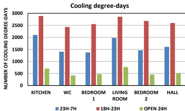
Figure 8 - Cooling degree-days for the cooling season (simulations performed without using fixed openings for ventilation in the facades)
