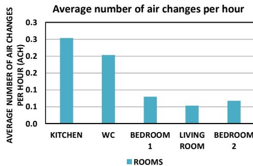
Figure 9 – Average number of ACH in the period of the heating season, for a simulation performed without using fixed openings in the facades
