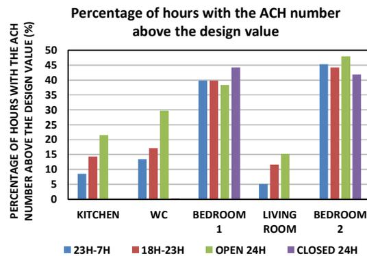
Figure 4 - PHAD for the cooling season (simulations performed using fixed openings for ventilation in the facades)
