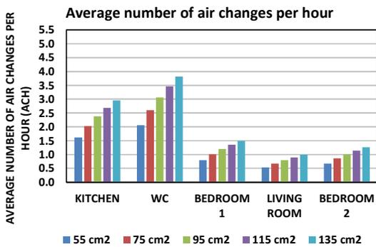
Figure 14 - Average number of ACH in the heating season for the simulations performed using zero wind speed
