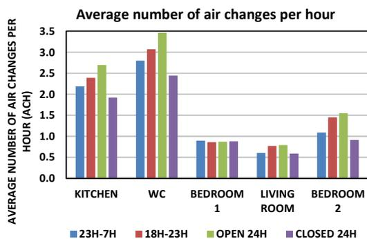
Figure 3 - Average ACH for the cooling season (simulations performed using fixed openings for ventilation in the facades)
