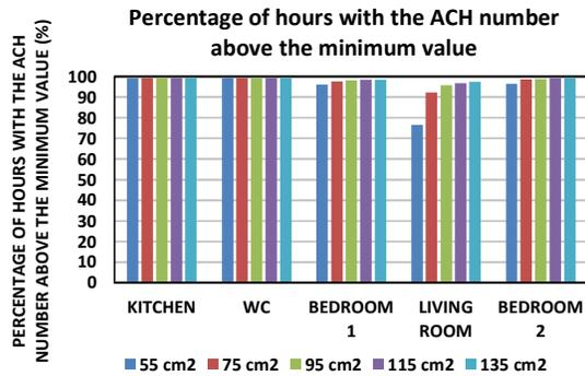
Figure 12 - PHAM in the heating season for the simulations performed using the wind speed according to the *Weather file*
