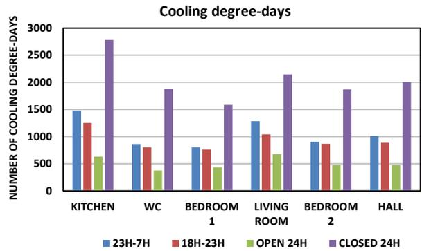
Figure 5 – Cooling degree-days for the cooling season (simulations performed using fixed openings for ventilation in the facades)
