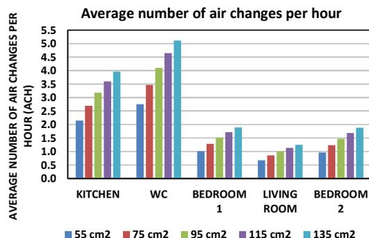
Figure 10 - Average number of ACH in the heating season for the simulations performed using the wind speed according to the *Weather file*
