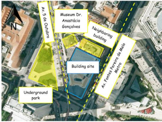
Figure 4: Representative scheme of neighbouring structures and services.
