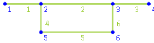
Figure 4.6 – Discretization of the cross-section into natural nodes and wall segments (extracted from GBTUL).
