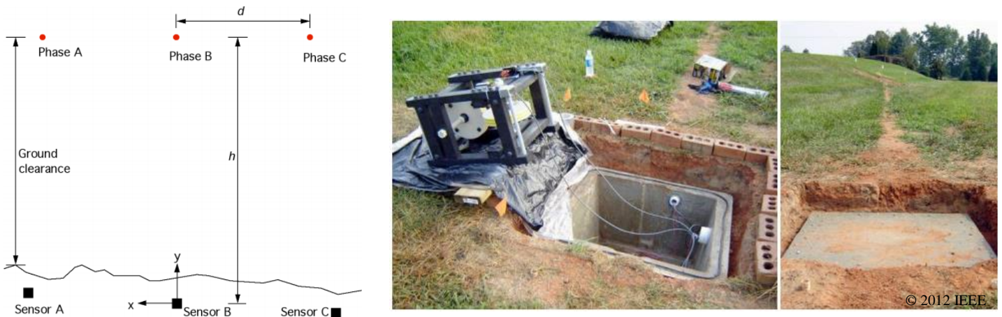
Figure 20: Promethean sensor position and burial [38].
