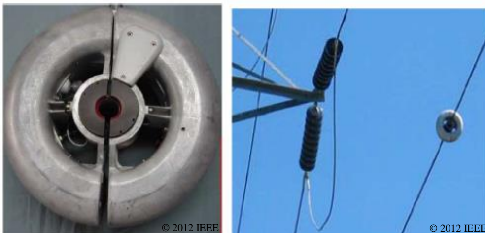
Figure 21: PD layout (left) and line installation (right) [38].
