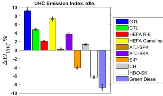
Figure 12:  $\Delta EI_{UHC}$  for Idle operating condition.
