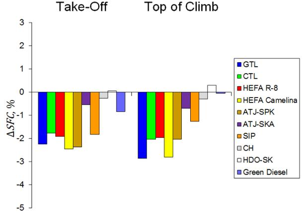
Figure 6: Summary of  $\Delta SFC$  for Take-Off and Top of Climb operating conditions.
