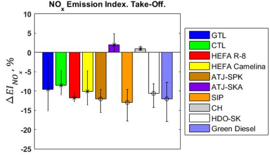
Figure 9:  $\Delta EI_{\text{NO}_x}$  for Take-Off operating condition.
