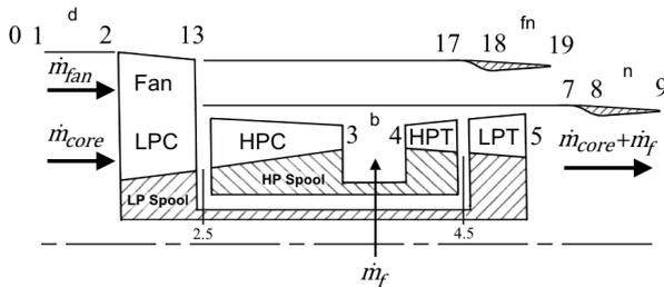
Figure 1: Two-spool turbofan station numbering ([9], adapted).
