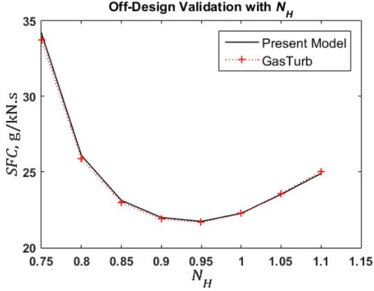
Figure 4: Off-design validation of specific fuel consumption,  $SFC$ , for given high-pressure relative spool speed,  $N_H$ .
