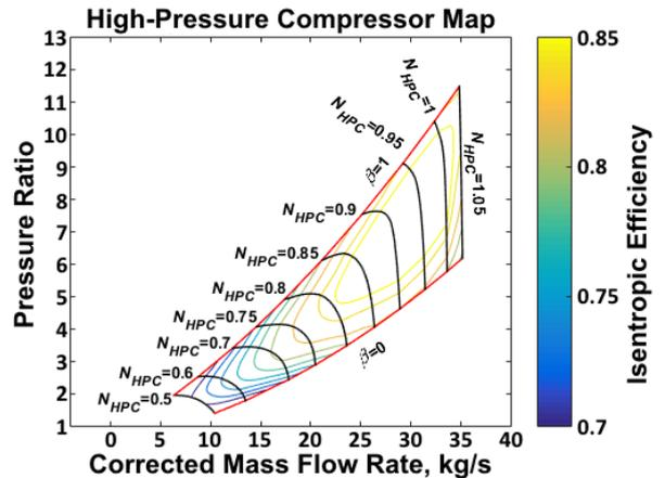
Figure 2: High-pressure compressor unscaled map. Based on data from [7].
