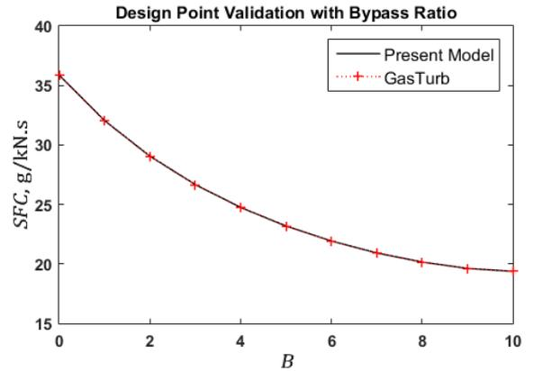
Figure 3: Design point validation of specific fuel consumption,  $SFC$ , with bypass ratio,  $B$ .
