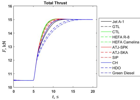
Figure 8: Total thrust,  $F$ , with elapsed time (acceleration), for fuel mass flow rate control.
