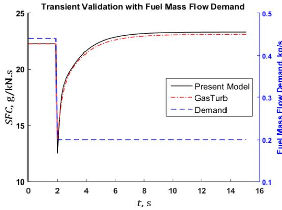
Figure 5: Transient validation of specific fuel consumption,  $SFC$ , with time,  $t$ , for  $\dot{m}_{f,demand}(t)$  input (deceleration).
