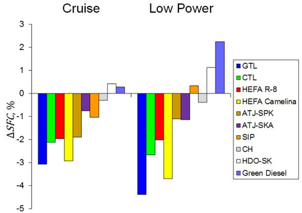
Figure 7: Summary of  $\Delta SFC$  for Cruise and Low Power flight conditions.
