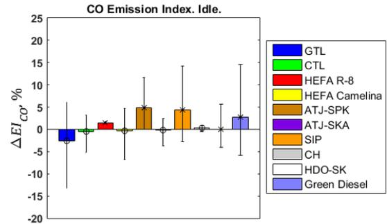
Figure 11:  $\Delta EI_{\text{CO}}$  for Idle operating condition.
