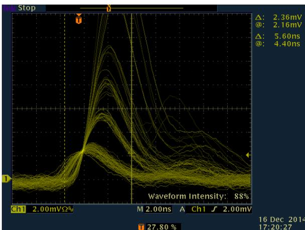
Figure 2: MPPC Hamamatsu S12572-50P The pulses have well defined amplitudes that multiple of the number of APD’s that discharged.
