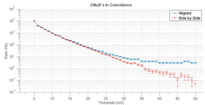
Figure 11: Measurement of two CMuD's in coincidence aligned and side by side.
