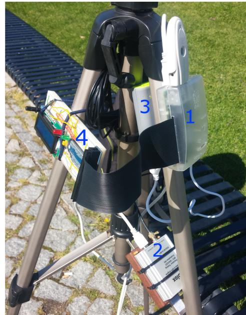
Figure 2: The solution developed for portable data collection: 1: Raspberry Pi and Wi-Fi adapter. 2: u-blox receiver. 3: Portable battery pack. 4: Breadboard with the LCD screen, button and LED's. The GPS antenna is not visible and sits at the top of the tripod, where a camera would usually be.
