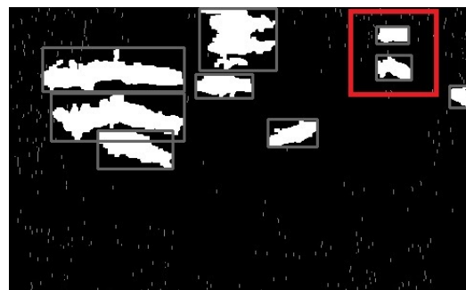
Figure 4.21: Frame to analyse with one fish mirroring at the top of the tank.
