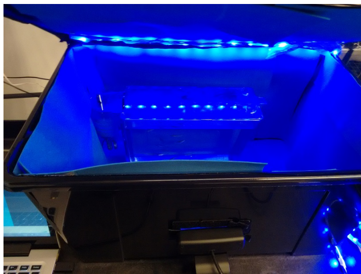
Figure 4.1: First version of the Danio Recording Setup with external USB webcam.
