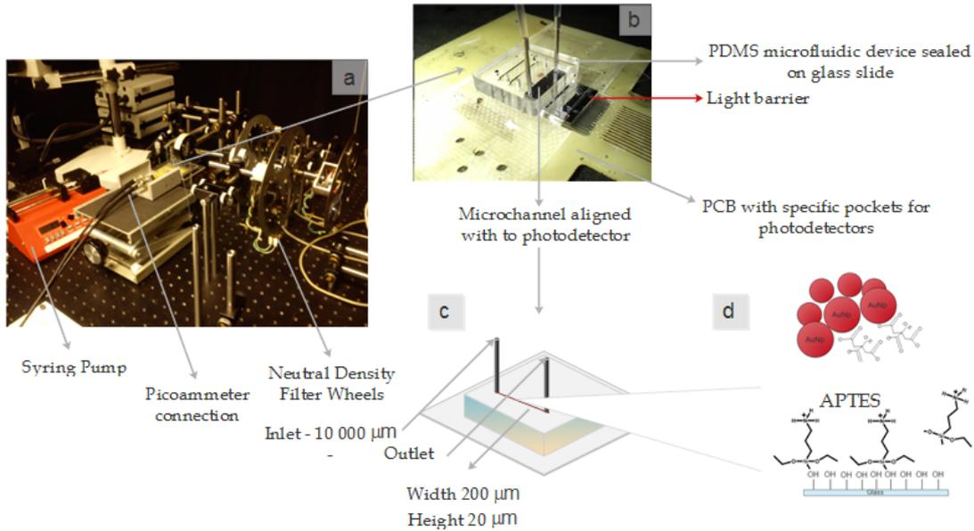
Figure 1: Photodetector integration for LSPR detection. a) Photograph of the optic apparatus for acquisition. b) Photograph of the PDMS microfluidic channels aligned to the light barrier and to the photodetector setup. c) Schematic of straight microfluidic channel used for LSPR detection. d) Illustration of the immobilization assay.
