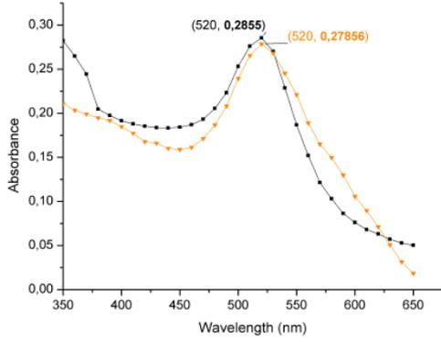
Figure 4: Comparison of absorbance values between the peak obtained by spectrophotometer (black curve) of colloidal AuNPs and the peak obtained by photodiode (orange curve), with immobilized AuNPs within the microfluidic channel after a 75 min assay.
