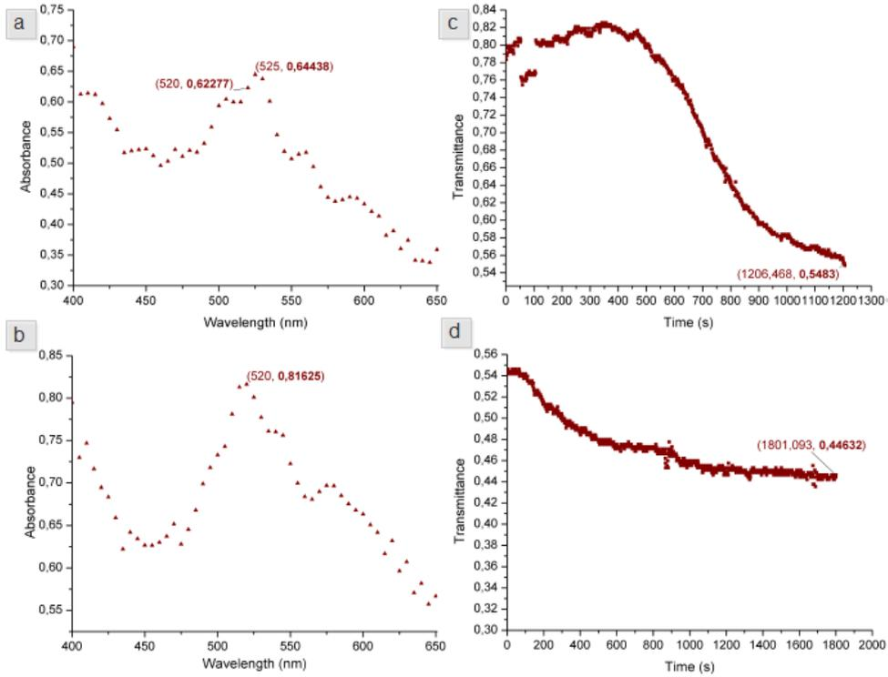
Figure 5: Photodiode acquisitions using ND3 filter and Al barrier aligned on top of the device. a) Absorbance spectrum after 20 min of AuNPs immobilization. b) Absorbance spectrum after 20+30 min of AuNPs immobilization. c) Transmittance over time of the first 20 min of flowing AuNPs. d) Transmittance over the following 30 min of flowing AuNPs.
