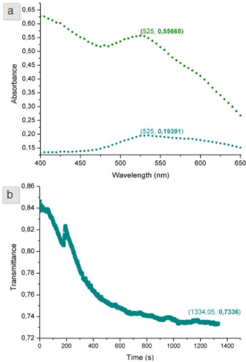
Figure 6: Photoconductor acquisition using an external applied voltage of 10 V, ND 0 filter and Al barrier. a) Absorbance spectrum of 30 min immobilization experiment (blue), compared with the yield absorbance spectrum after BSA was flowed into the same channel (green). b) Transmittance over the 30 min of flowing AuNPs into the microfluidic channel.
