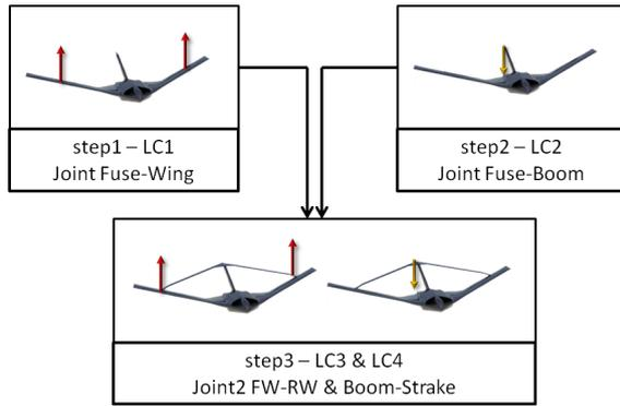
Figure 6: Steps for the optimization of the Joints on the Sensorcraft.
