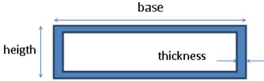
Figure 9: Hollow Cross Section.
