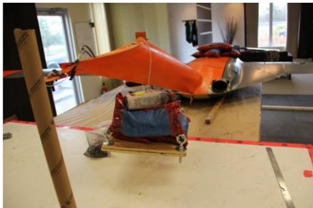
Figure 3: Static Test Boom Load.
