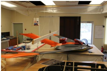
Figure 2: Static Test Forward Wings Load.
