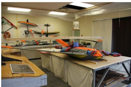
Figure 4: Static Test with Aft Wings, Wing Load.
