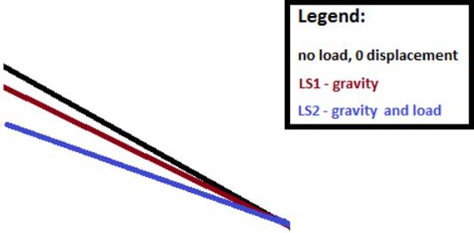
Figure 2.8 - Scheme of the boom displacement for both load steps
