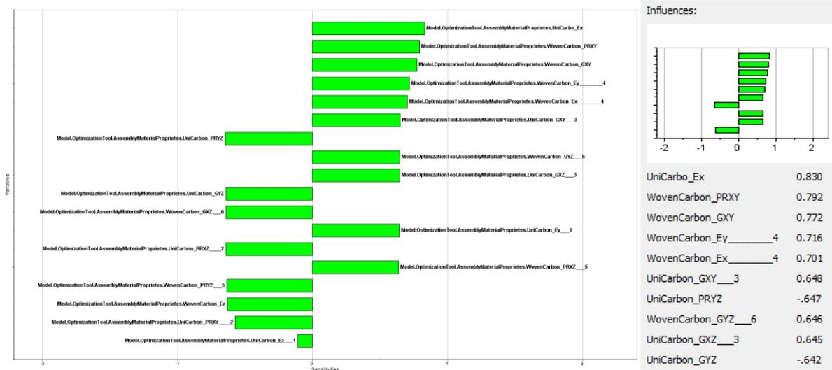
**Figure 2.17 - Sensitivity study of the material properties for Carbon Fiber Woven and Unidirectional**
