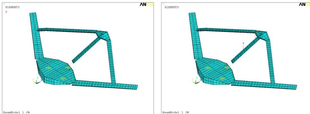
**Figure 4.2 – Beam model Fuse Load (left) and Boom Load (right)**
