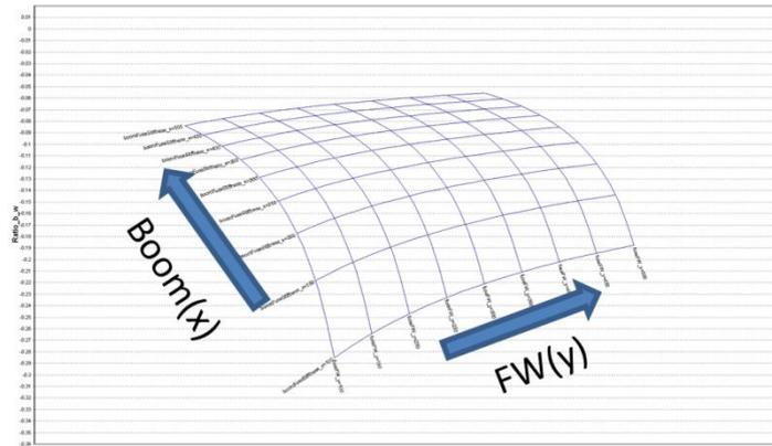
**Figure 4.18 – Carpet plot of the FW(y) and Boom(x) joints with the response of the ratio between boom and FW deflections**
