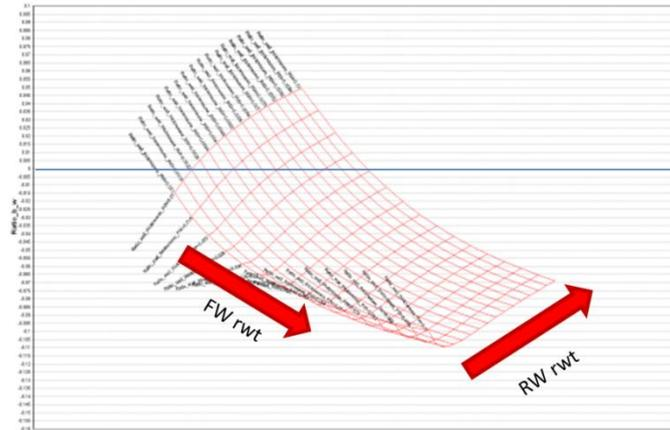
**Figure 4.20 – Carpet plot of the FW and RW ratio wall thickness with the response of the ratio between boom and FW deflections**
