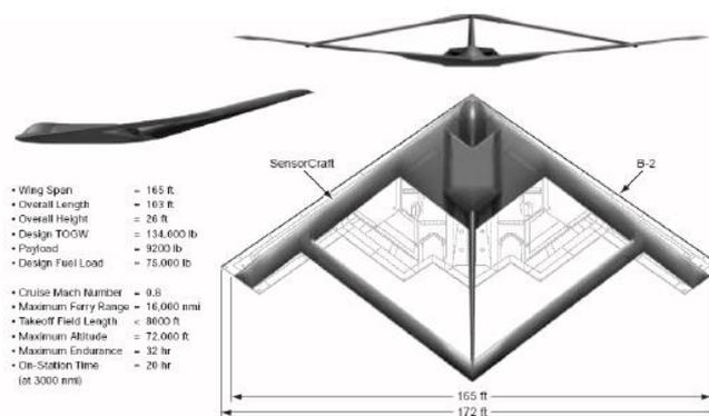
Figure 1.7 - Boeing™ SensorCraft view and comparison size with B-2 [3]
