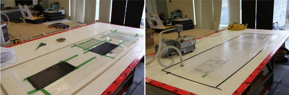
Figure 2.13 - Lamination of the rectangular shape of coupons (left) and the vacuum bag (right)
