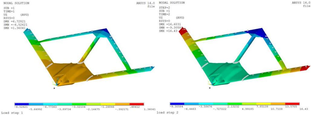
**Figure 2.9 - High Fidelity Model: displacement plots [mm] for both load steps with load on wings, LS1 (LHS), LS2 (RHS)**
