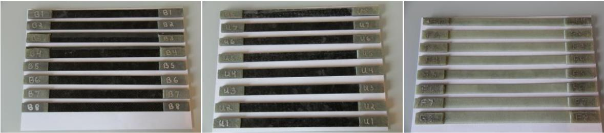
**Figure 2.15 - Test specimens, carbon fibre woven (left), carbon fibre uni-directional (mid), glass fibre woven (right)**
