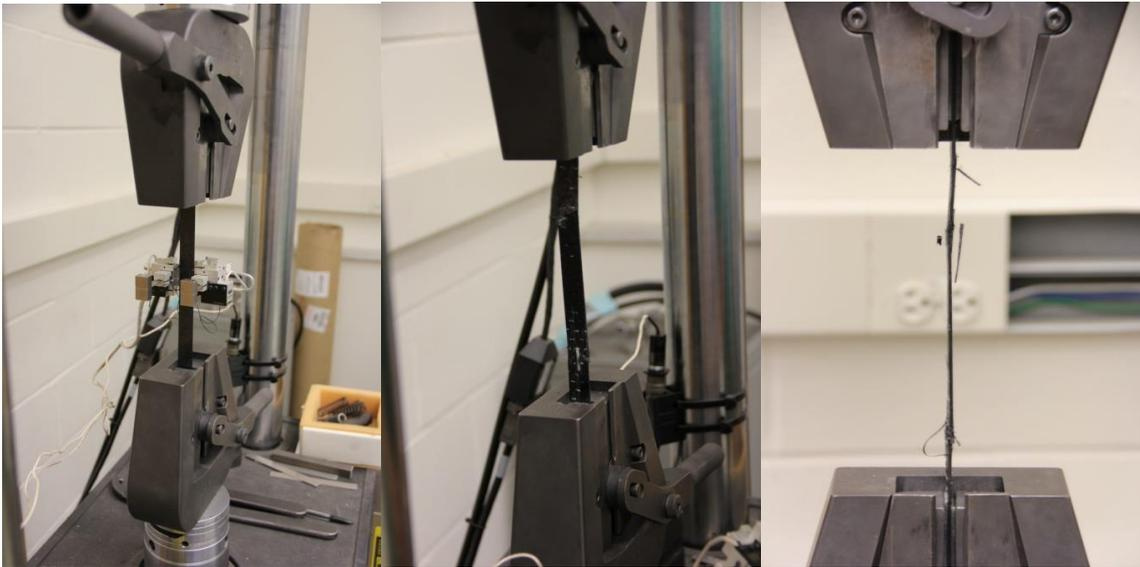
**Figure 2.16 - Tensile Tests at different angles**
