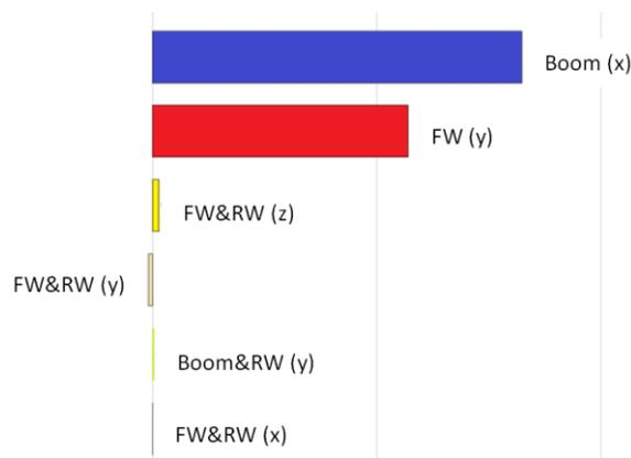
**Figure 4.11 - Sensitivity Study for joints regarding boom deflection**
