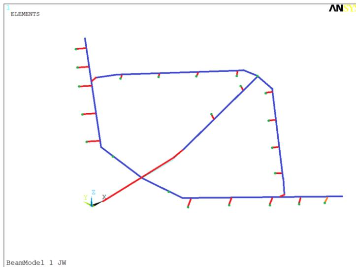
**Figure 3.5 - Beam Model with rigid element to transfer the force at 0% of chord**
