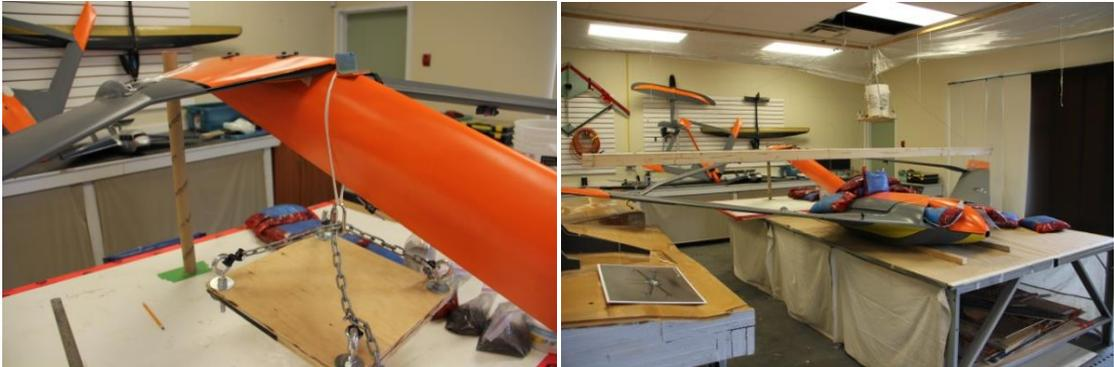
Figure 2.3 - Static Test with Aft Wings, Boom Load (left), Wing Load (right)
