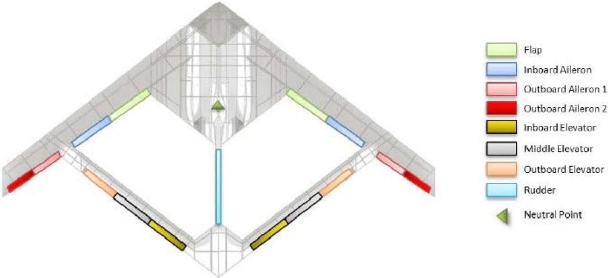
**Figure 1.4 - Control surfaces of JWSC [7]**
