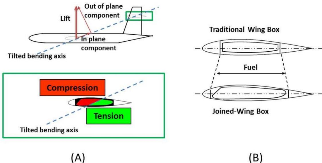
Figure 1.6 - (A) Tilted bending axis of joined wing configuration; (B) Wing Box Comparison [4]
