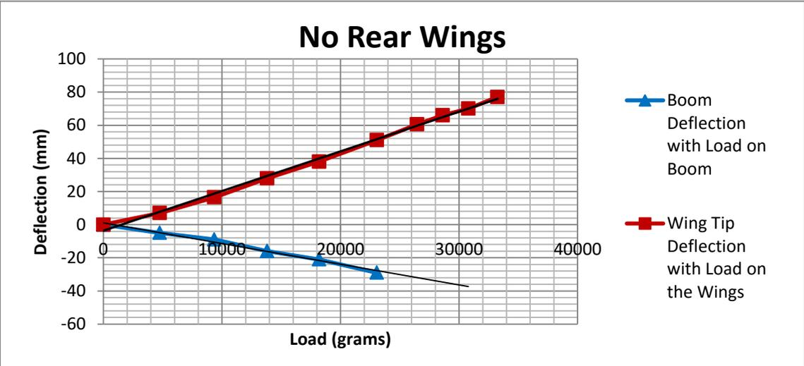
Figure 2.4- Results for the Static Test without the Aft Wings
