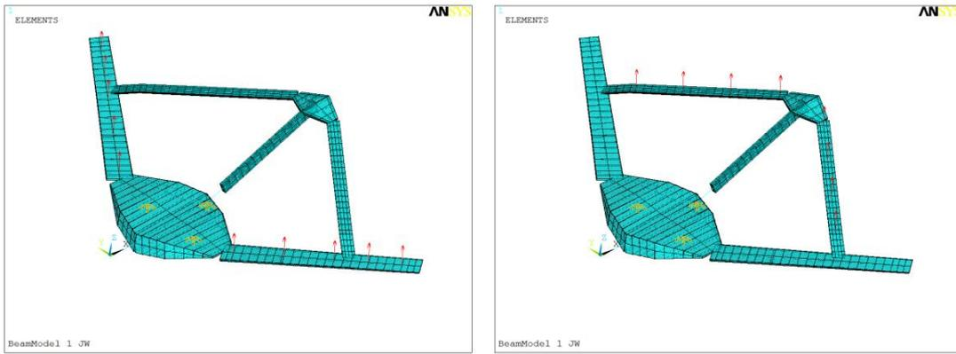
**Figure 4.3 – Beam Model Forward Wing Load (left) and Aft Wing Load (right)**
