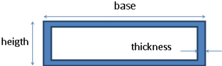
**Figure 3.8 - Hollow Cross Section**
