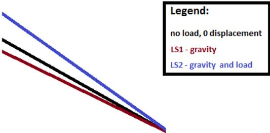
Figure 2.7 - Scheme of the forward wing displacement for both load steps
