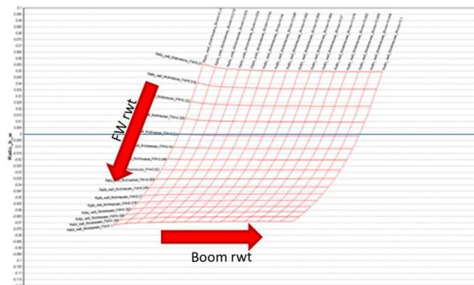
**Figure 4.21 – Carpet plot of the FW and Boom ratio wall thickness with the response of the ratio between boom and FW deflections**
