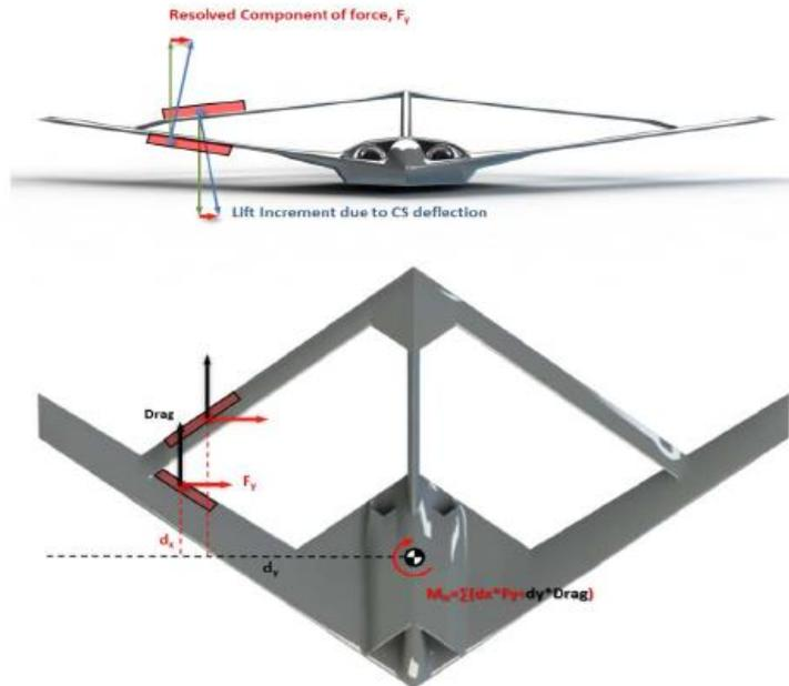
Figure 1.5 - Effect of resolved lift increment on aircraft yaw [7]
