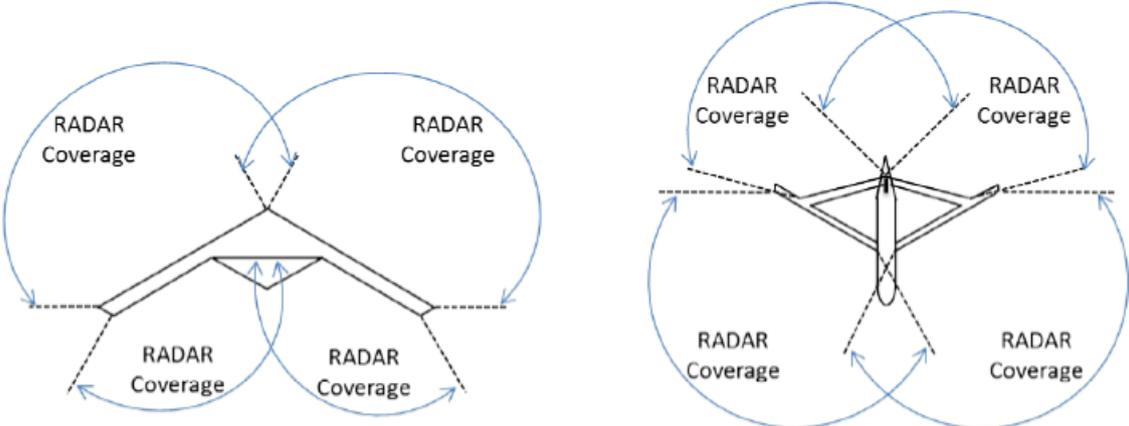
**Figure 1.3 – Sensor packages on conventional wing and Joined Wing [2]**
