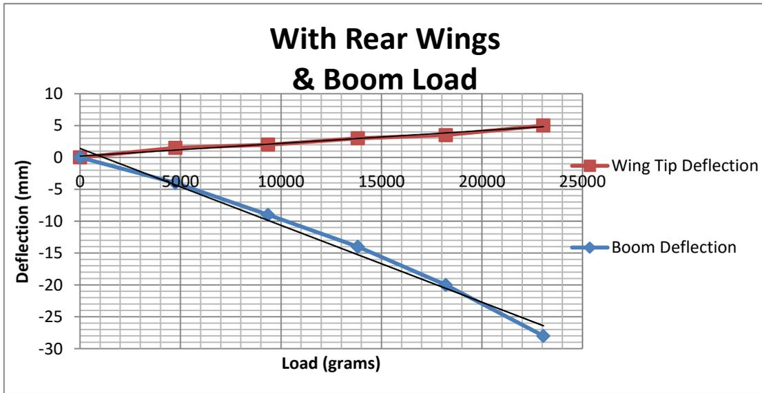
Figure 2.5 - Results for the Boom Load with Aft Wings
