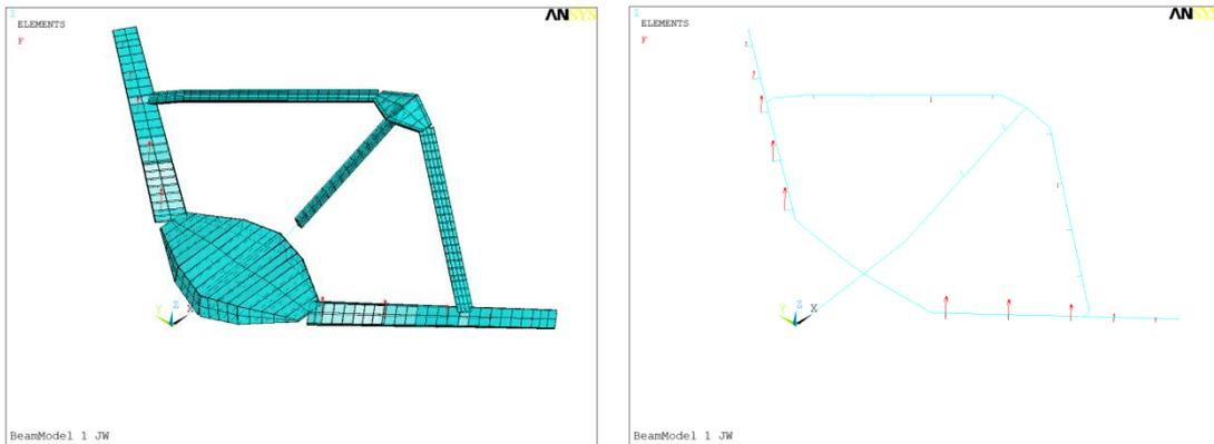
**Figure 4.4 – Beam Model Full Wings Load (left - beams shape; right– 1D elements)**
