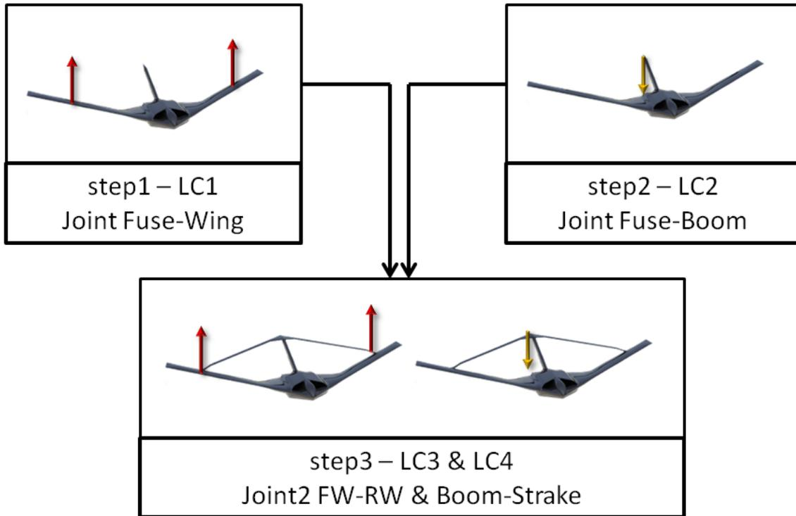
Figure 2.11 - Steps for the Optimization of the Joints on Sensorcraft
