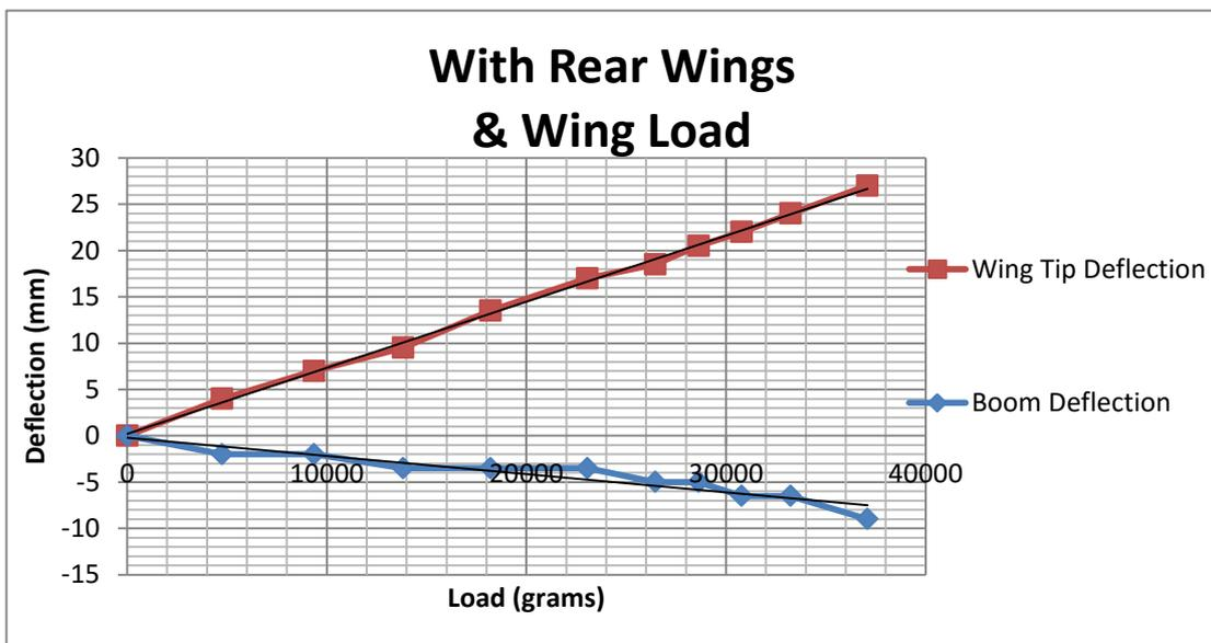
Figure 2.6 - Results for the Wing Load with Aft Wings
