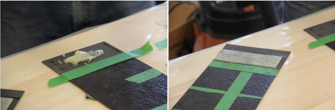
Figure 2.14 - Adhesive of fibre glass tabs in the rectangular shape
