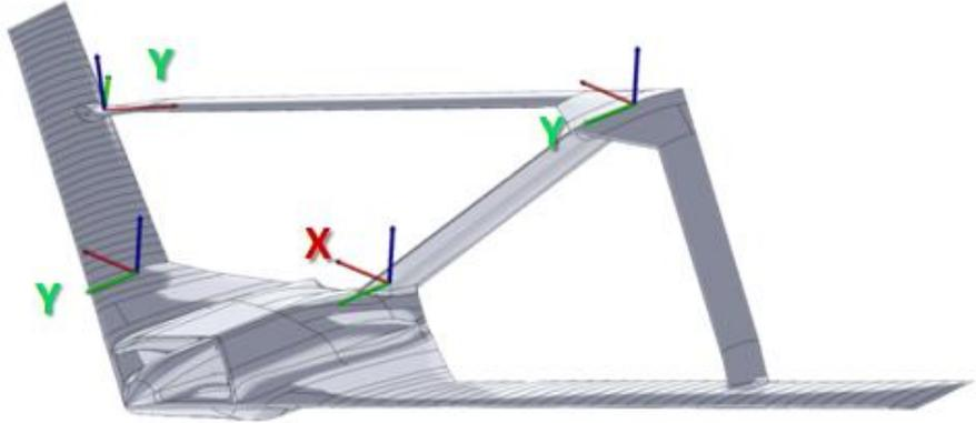
**Figure 3.7 - Original CAD model with the allowable joints rotations**
