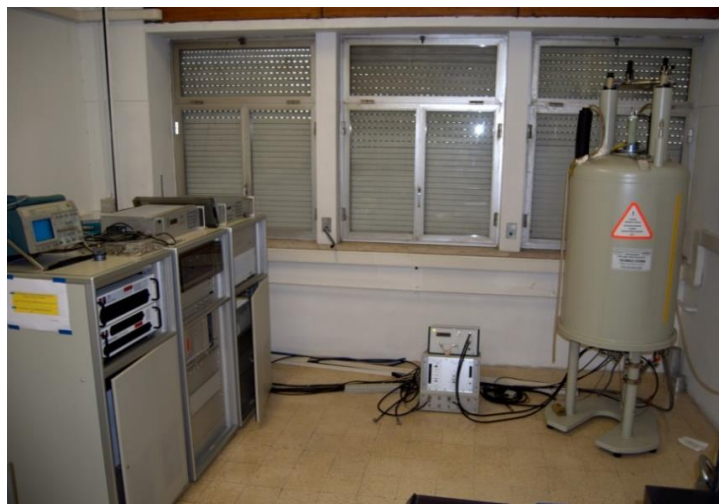
Figure 17: ^{13}\text{C} NMR spectrometer Bruker Avance 300 MHz used in IST-UL NMR lab.
