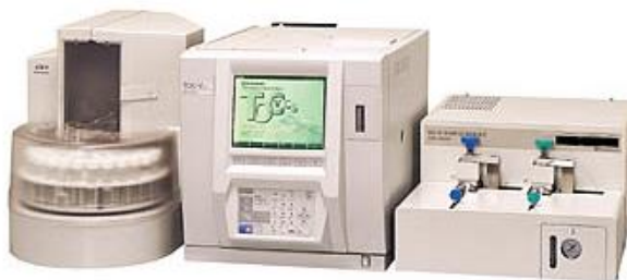
Figure 11: Shimadzu TOC 5000A instrument used for the HTOC analysis.
