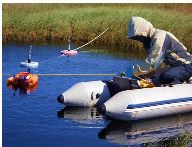
Figure 9: Water collection on SAS 2A Lake using a pump with a graded hose.
