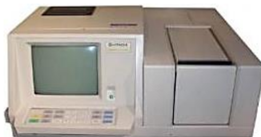
Figure 15: Hitachi-2000 spectrophotometer used for the sulfate analysis.
