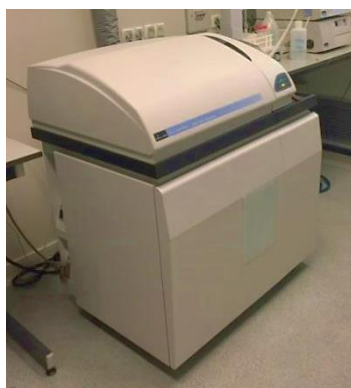
Figure 21: ICP-MS filter quadrupole mass of ELAN DRC-e Perkin Elmer used on this work (C 2 TN).
