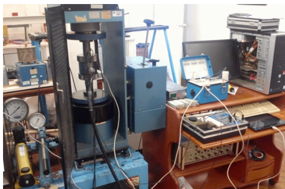
Figure 2 – Apparatus for the triaxial rock test with stress, strain, P-wave and S-wave measurements.
