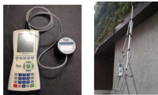
Figure 8: Presentation (Fernandes, 2014) and installation of Isomet 2114
