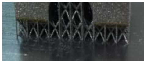
Figure 43 – Lattice structures implemented in the support study.
