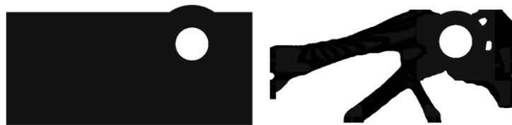
Figure 2 – Right plane view on a 3D TO initial design domain and solution
