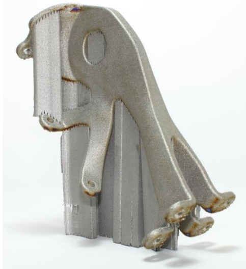
Figure 52 – Optimised component with supports. STL file (left) and component after being removed from the platform (right).
