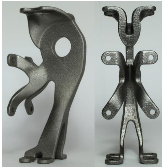
Figure 53 – Optimised component after the support structures removal.
