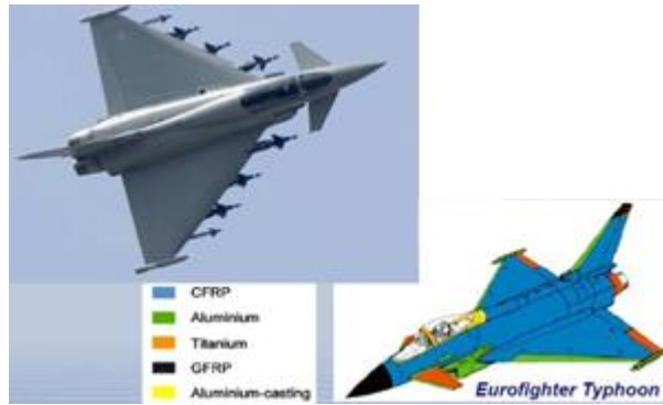
Figure 13. Distribution of composite materials in Eurofighter Typhoon [12]
