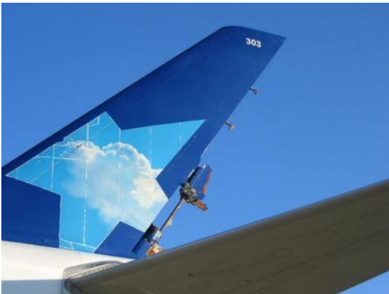
Figure 6. Different views of the detachment of the rudder of Air Transat flight [6]
