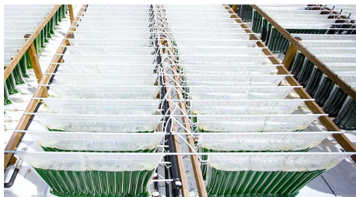
Figure 2.14. Algenol's 2 nd generation PBR design. [Adapted from (46)].
