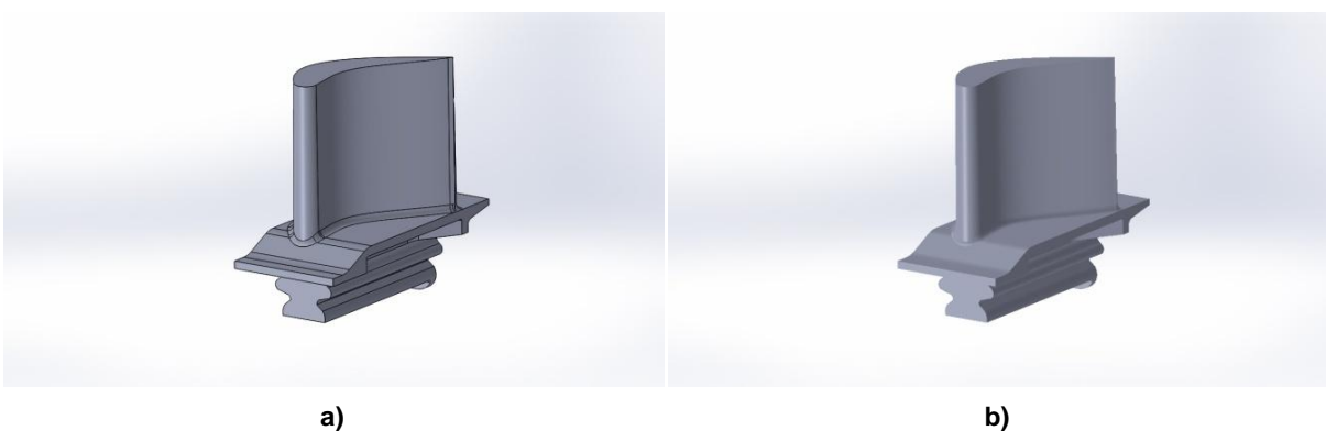
Figure 3.11 – a) HPT blade 3D model a) with drawing edges; b) without drawing edges.
