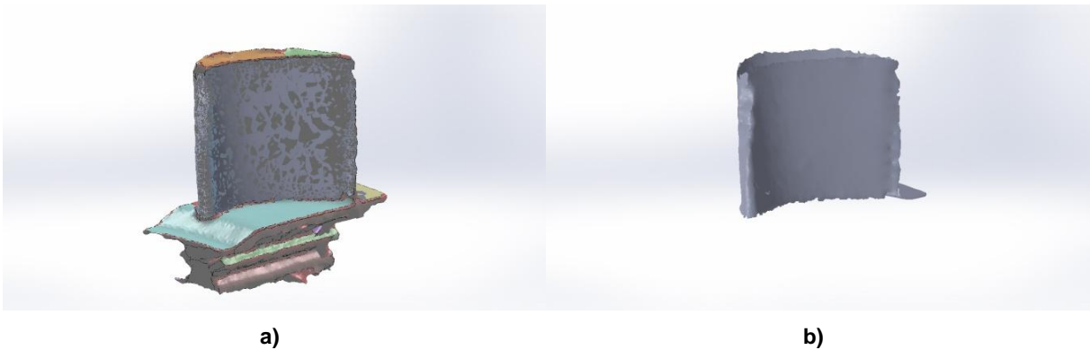
Figure 3.10 – a) Polygon mesh of part surface; b) editable surface of part.
