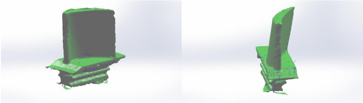
Figure 3.9 – 3D surface mapping of the HPT blade scrap in the ZScan software.
