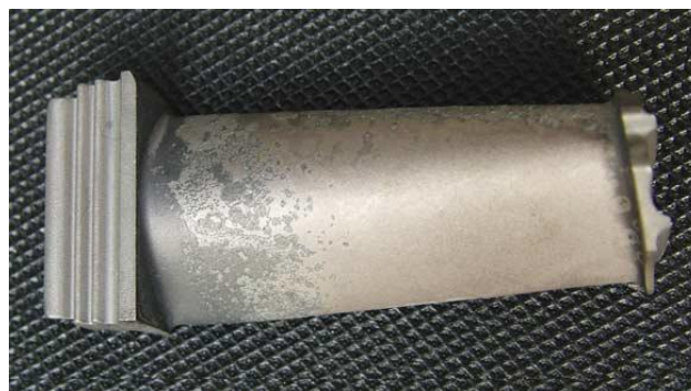
Figure 2.24 – Sulphidation attack of a turbine blade. [47]
