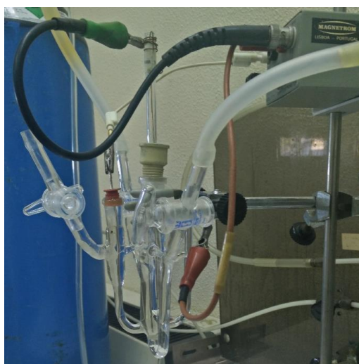
Figure 2.3 A three electrode system with a Silver pseudo-reference electrode and a Platinum auxiliary- and working electrode.
