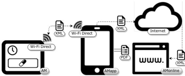
Figure 1: System's architecture for situations without permanent access to the Internet.
