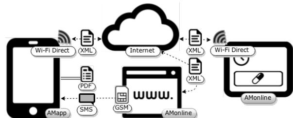
Figure 3: System's architecture for a solution with constant access to the Internet.
