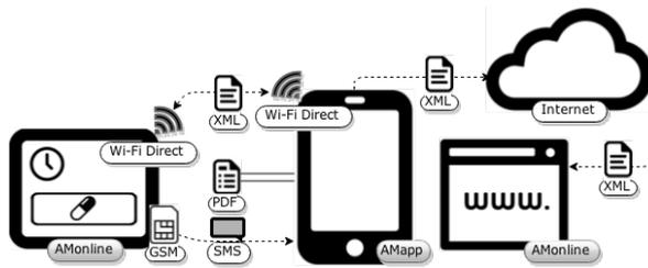
Figure 2: System's architecture for situations without permanent access to the Internet but with cellular mobile communication.
