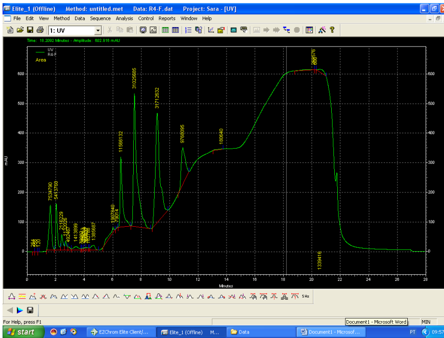
Figure 26 Chromatogram for the injection of IME4 samples from R4: a) time zero b) after 48 hours.
