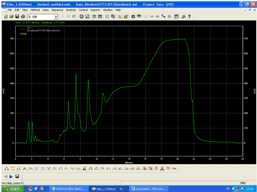
Figure 19 – Typical chromatogram for the injection of a sample of butyl oleate in reversed micelles reaction media.
