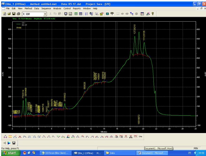
Figure 23 Chromatogram for the injection of control samples from R3: a) time zero b) after 48 hours.
