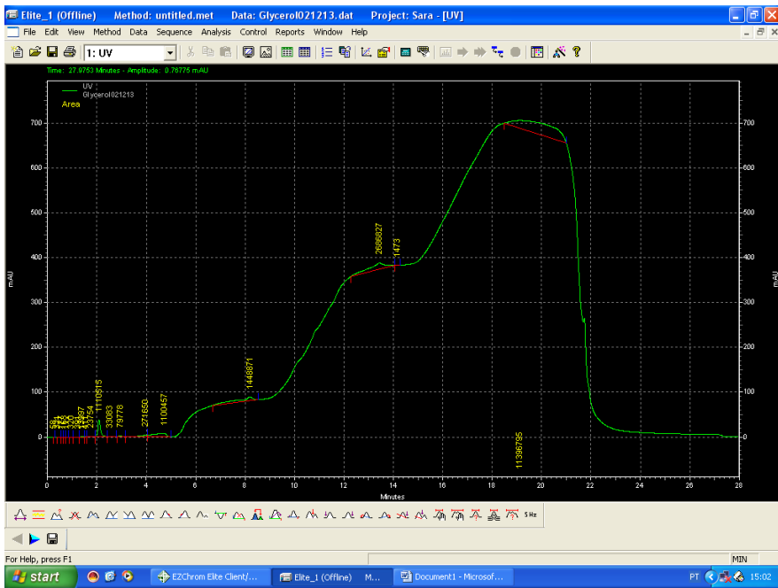
Figure 18 – Typical chromatogram type for the injection of a sample of Glycerol diluted only in n-hexane.
