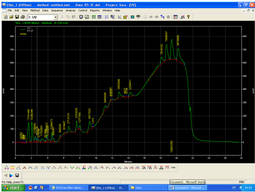
Figure 25 Chromatogram for the injection of IME3 samples from R3: a) time zero b) after 48 hours.
