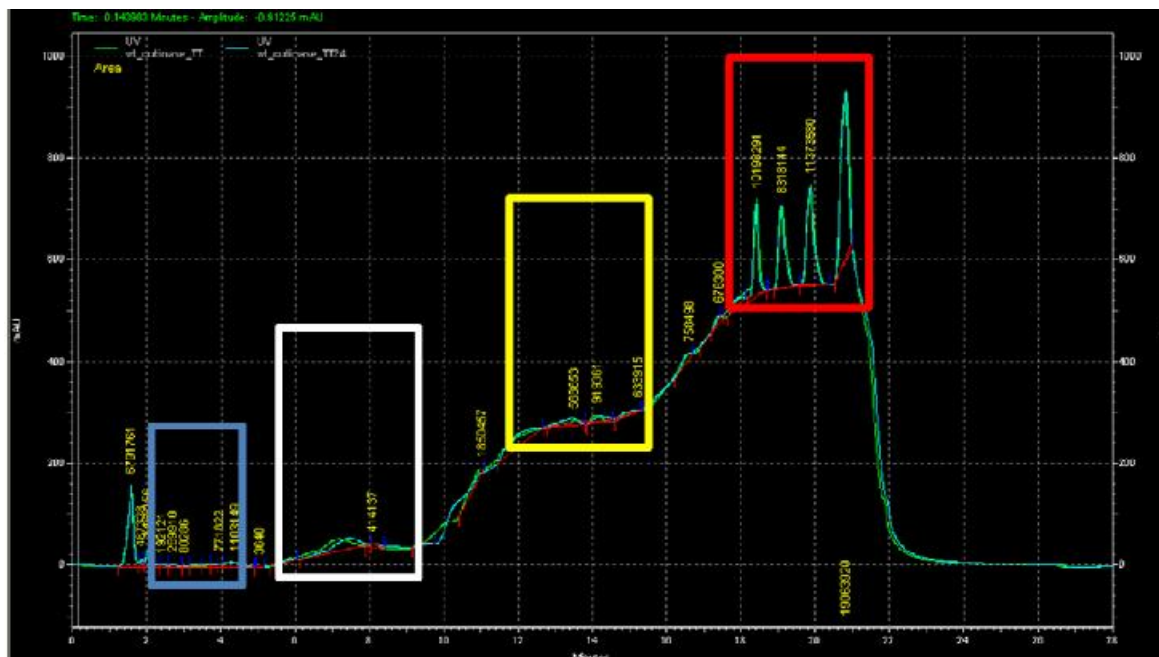
Figure 20 Resume of typical chromatogram and the time zone of substrates, intermediates and products. Blue rectangle – time zone of MG detection, White rectangle – time zone of Alkyl Esters detection, Yellow rectangle – time zone of DG detection, Red rectangle – time zone of TG detection.
