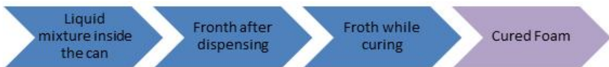
Figure 3.1: Schematic diagram of foaming process.
