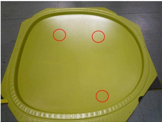
Fig. 3.– Example of typical anomalies found in a Pressure dome, 3 scratches on the inner face.
