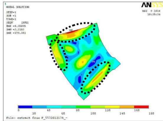
Fig. 11. – Edges stress concentration at outer face thickness decrease of 10%, on inner face.
