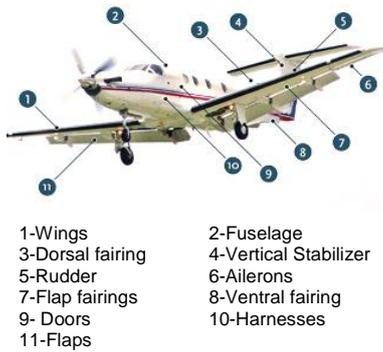
Fig. 1 – Pilatus PC-12. *Courtesy of OGMA*
