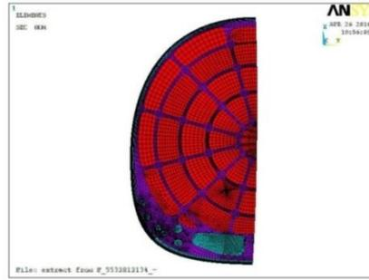
Fig. 6. – Thickness decrease analysis mesh, modified area identified in blue at the right picture.
