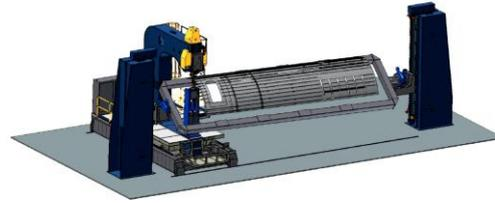
Fig. 12 – Component being riveted by an automatic fastening machine. *Courtesy of Gemcor*
