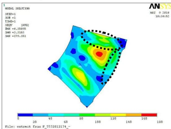
Fig.10. – Edges stress concentration at outer face thickness decrease of 10%, on outer face.
