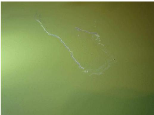
Fig. 4. – Scratch example. Courtesy of OGMA
