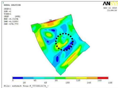
Fig. 9. – Von-Mises stress distribution for same thickness decrease at outer face.
