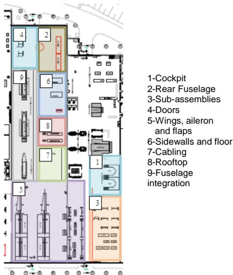
Fig. 2 – Pilatus PC-12 Production Line, FMT Layout. *Courtesy of OGMA*
