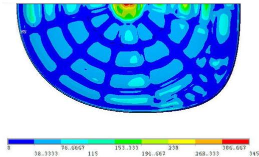
Fig. 5– Von Misses Equivalent Stress plot of outer face.
