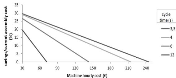
Fig. 13 – Profitability analysis of LH and RH PC-12 sidewalls riveting automation.
