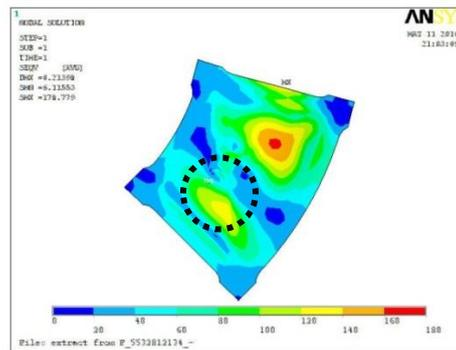
Fig. 8. – Von-Misses stress distribution for inner face thickness decrease of 25% at inner face, using refined mesh.
